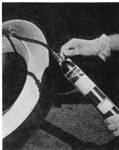
Tire inflated in four to ten seconds
