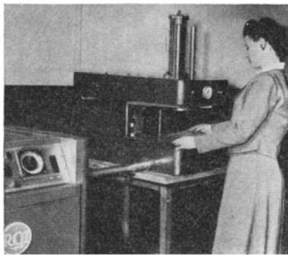
Thermoplastics sealer in operation
