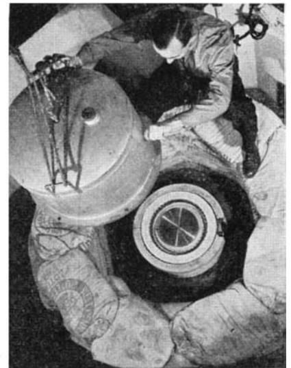
Looking down into the pit where new alloys are whirled to destruction
