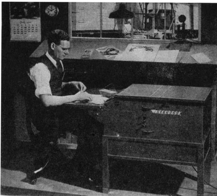
Lower left: At a busy freight terminal, a clerk inserts waybills into a machine which microfilms them at rate of 90 a minute Lower right: Another clerk, with a microfilm frame enlarged on a reader, picks out information for a bill or record of shipment
