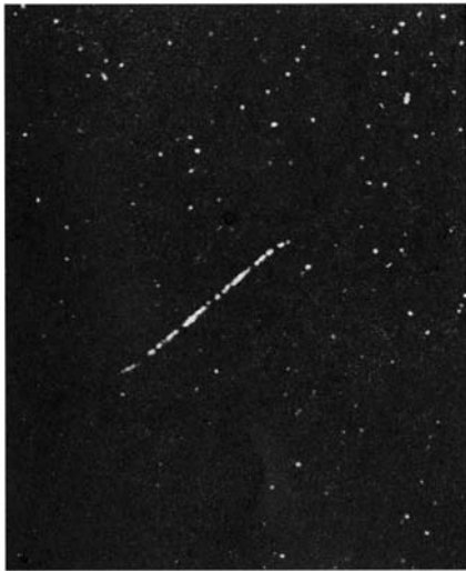
White streak marks the paths of two new atoms created by the fission of a uranium atom at midpoint of streak
