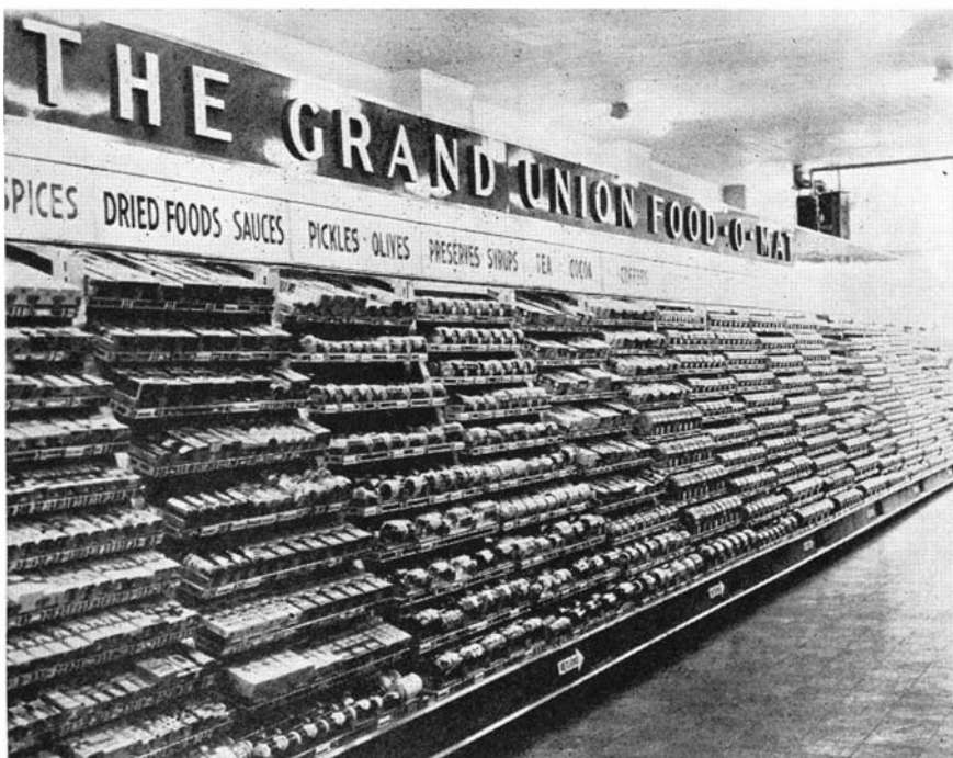
As soon as a package is removed from the rack, another slides down to take its place
