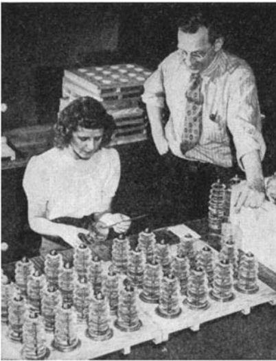
Glass bushings at final inspection
