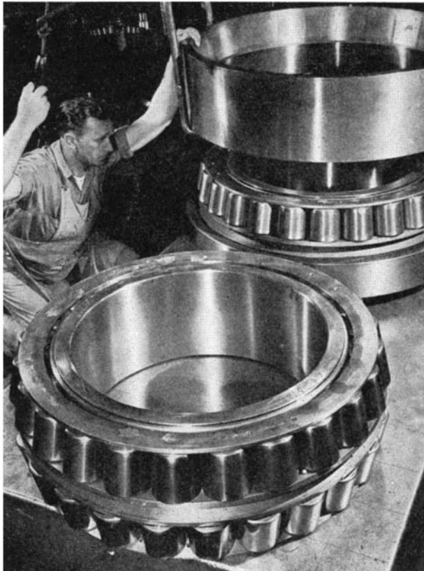
Roller bearings so large that a crane is used in assembling them
