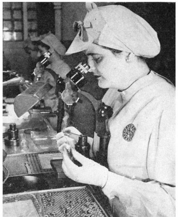
Air conditioning protects tiny bearings during assembly and inspection
