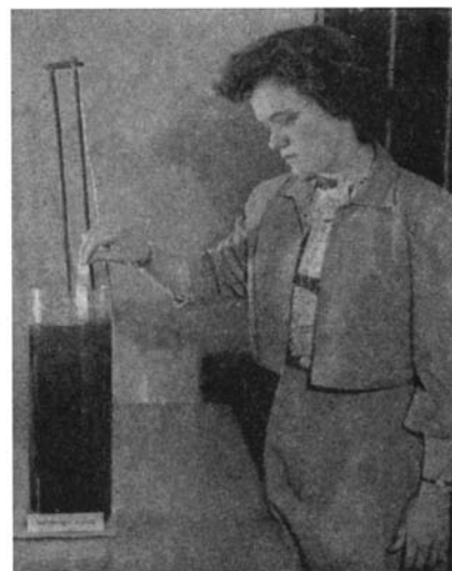
Equipment for electroless plating includes only vessel, solution, and immersion heater (projecting from bath)
