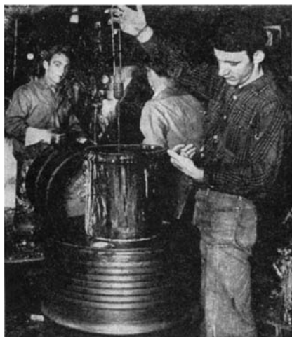
Measuring enamel's viscosity
