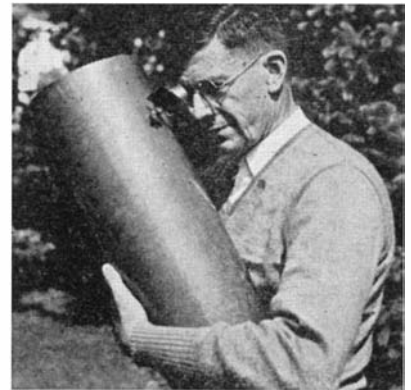
Richest-field telescope with eyepiece and auxiliary diagonal finding mirror
