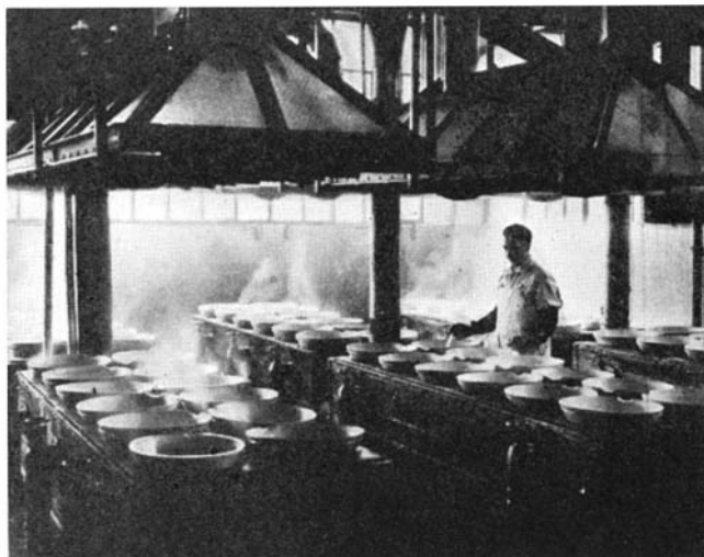
Producing a continuous stream of silver nitrate crystals, the new process (left) replaces the slow open-dish evaporation method (right)
