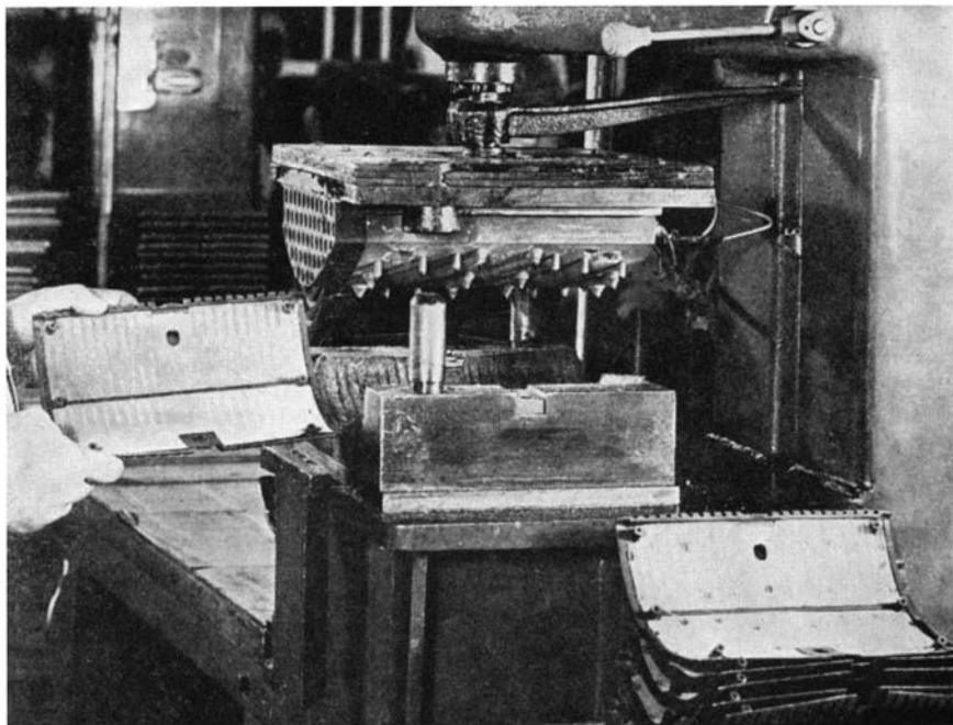
One such press can turn out 100 metal-plastics grills per hour
