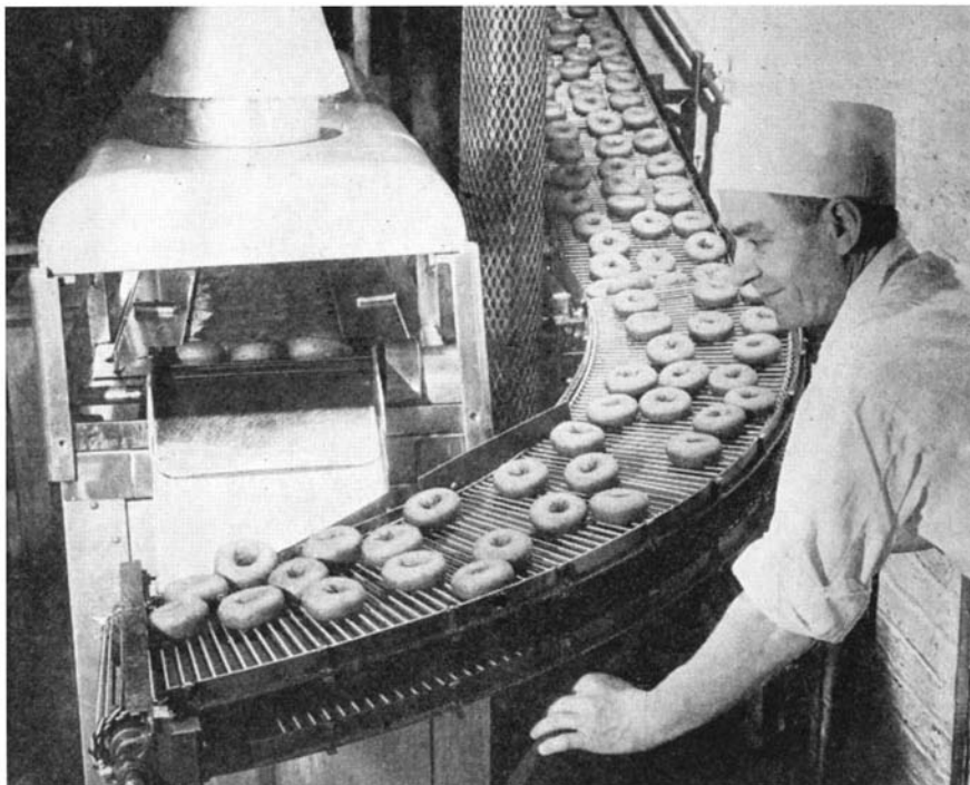
Open construction of the wire conveyor facilitates cooling of articles in transit
