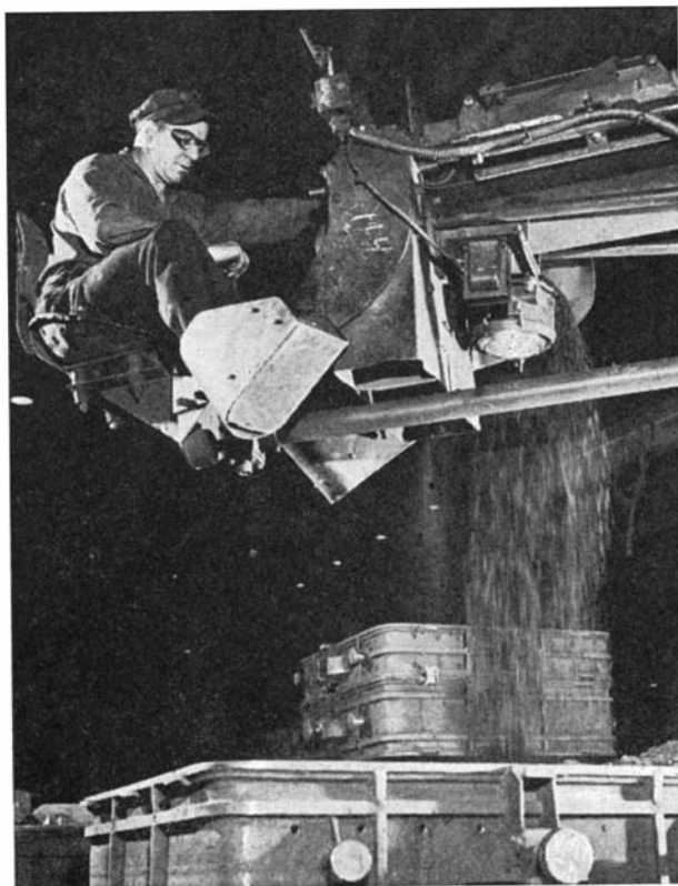
Replacing the traditional hand shovel, this “sandslinger” hurls 1000 pounds of sand a minute into the mold
