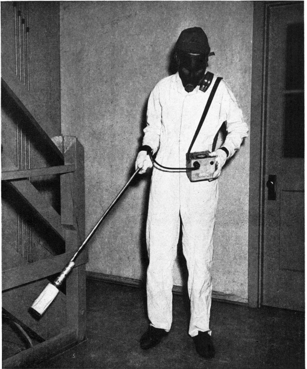
Completely swathed in protective clothing a health physics inspector measures radiation intensity with a fish pole meter
