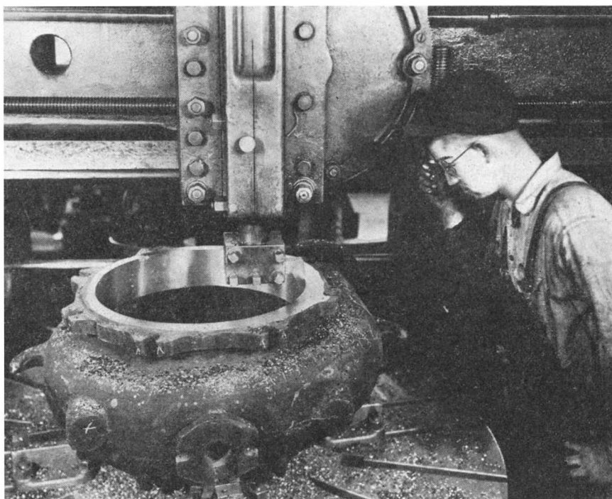
Rough cuts as heavy as .075 inch can be made
