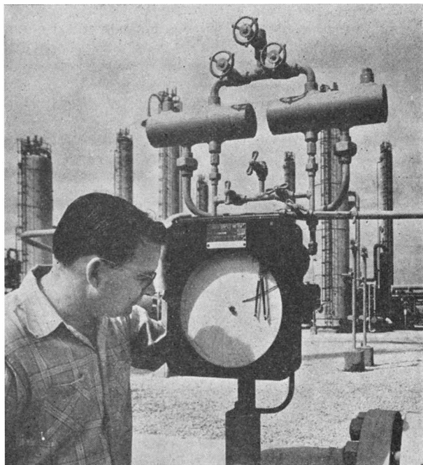
This gage records the pressure of the residue gas as it is forced back into the ground
