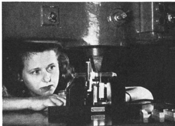
A laboratory technician measures the force required to break a sample of polystyrene on a physical testing machine
