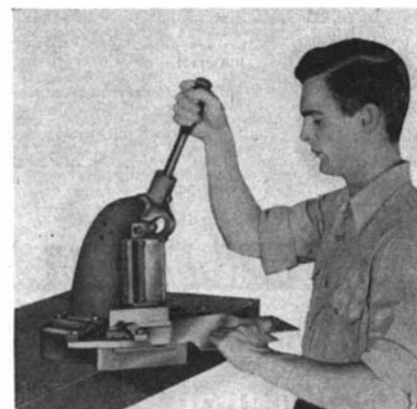
Notcher makes a clean, burr-free cut
