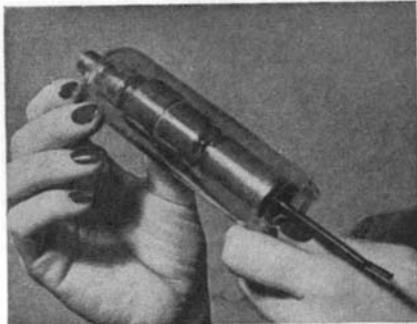
Small dental X-ray tube is built to operate for 20 years of normal service
