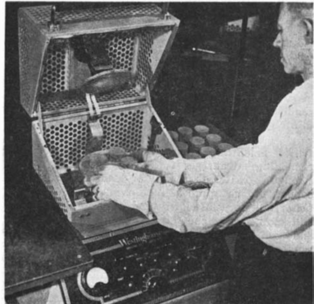
Placing plastics preforms in a dielectric heater. Dielectric heating cuts the cost of molded plastics and improves the quality of the product
