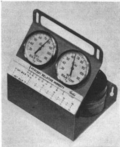
Indicator is accurate to \pm 1 per cent
