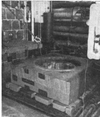
In this whirl pit circular steel plates are spun at high speed until they burst
