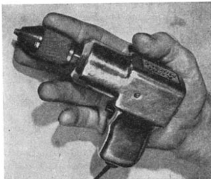
Power drill takes bits up to ¼ inch
