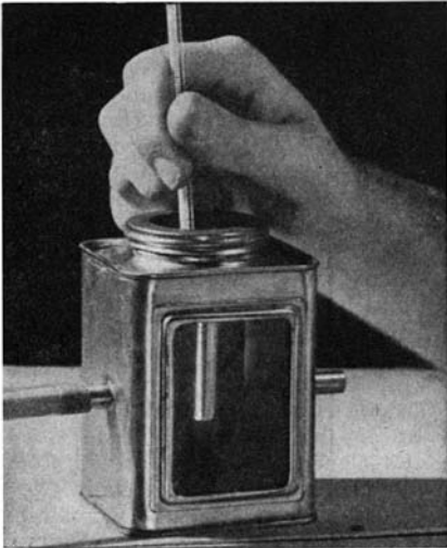
The apparatus determines dew points at temperatures as low as minus 76 degrees, C.
