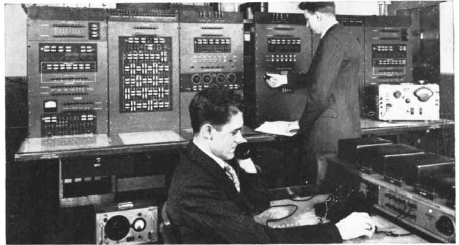
The engineer in the foreground talks over the test circuits which the other engineer sets up on a "circuit simulator."
