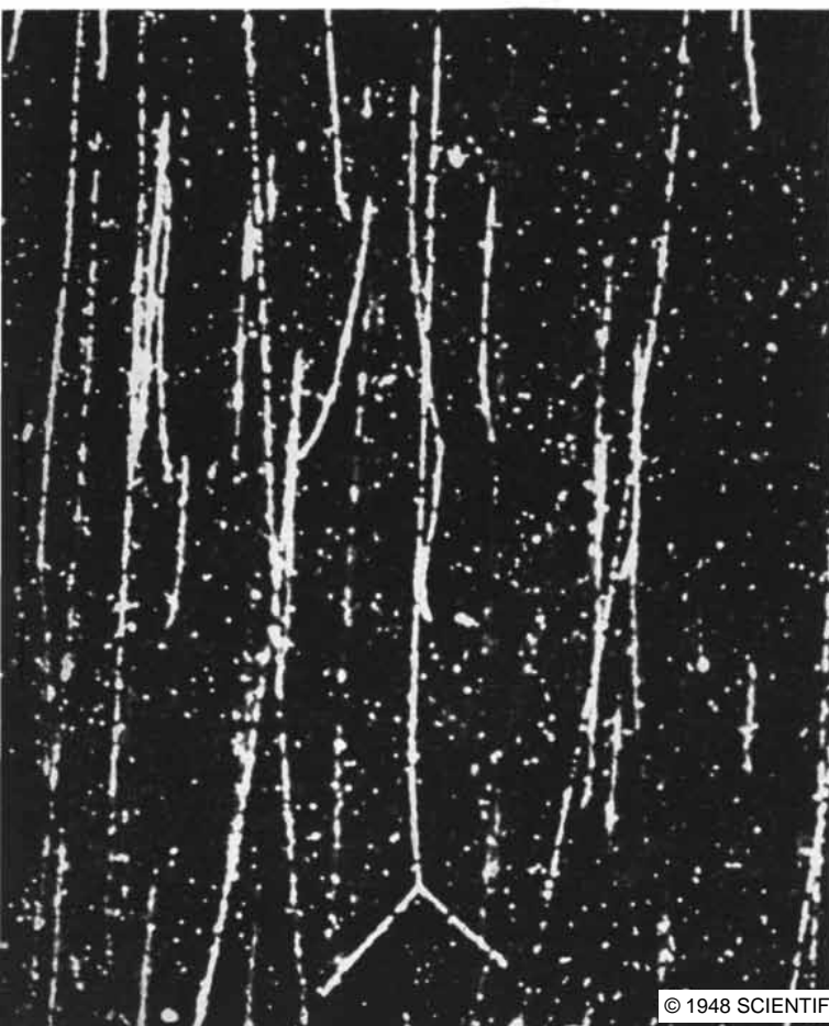
COLLISION of one proton with another is indicated by forked track at bottom. Bombarding proton is deflected at an angle; the other leaves a track in recoiling.
