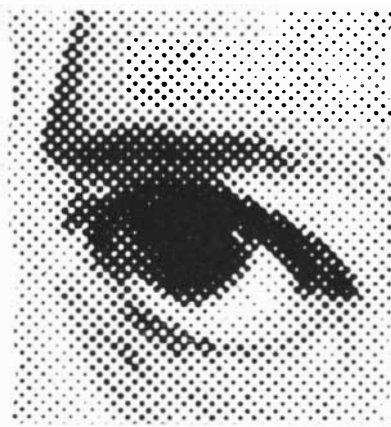
HALFTONE engraving, here enlarged, creates effect of shading with one ink and dots of various sizes.
