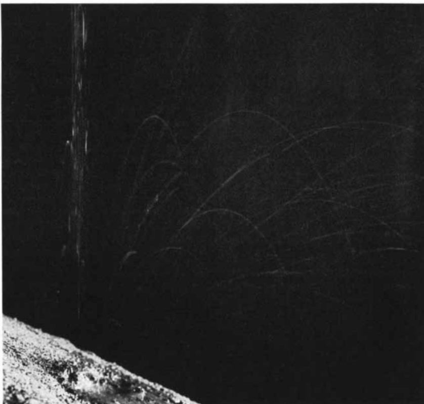
IMPACT AT AN ANGLE can move large quantities of soil downhill. This scalps topsoil from the crest and concentrates it at the bottom of the slope. Later the good soil may be buried by subsoil splashed down from above.
