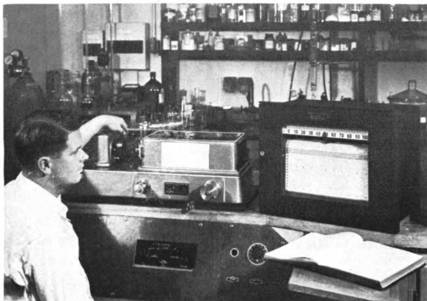
A Perkin-Elmer Infrared Spectrometer installed at the Hooker Electrochemical Company at Niagara Falls, New York. Here the instrument is an important link in the production of the insecticide Benzene Hexachloride.
