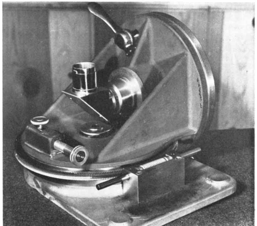
Porter-revised Springfield mounting cast in aluminum by Ensign
