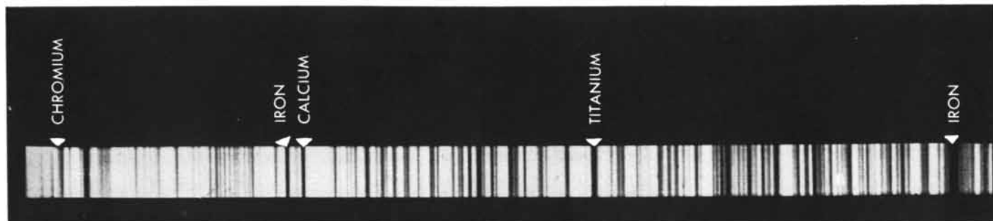
SPECTRUM OF THE SUN shows an intricate series of dark lines indicating the characteristic wavelengths ab-
