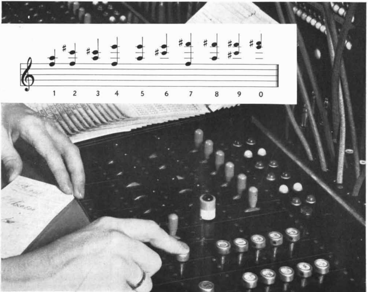
Above is the Bell System's new "musical keyboard." Insert shows the digits of telephone numbers in musical notation, just as they are sent across country.
