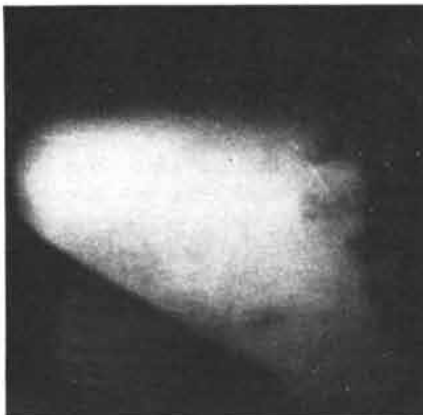
WATER VAPOR is supercooled in a tank during laboratory experiment in precipitation by dry ice crystals.
