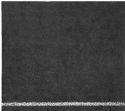
PURE TONE of 250 cycles a second appears as a single horizontal line.
