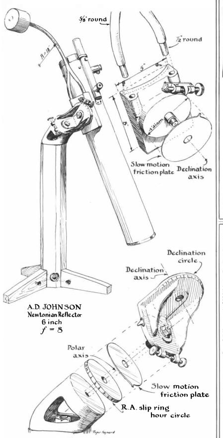
The Johnson portable semi-Springfield reflecting telescope
