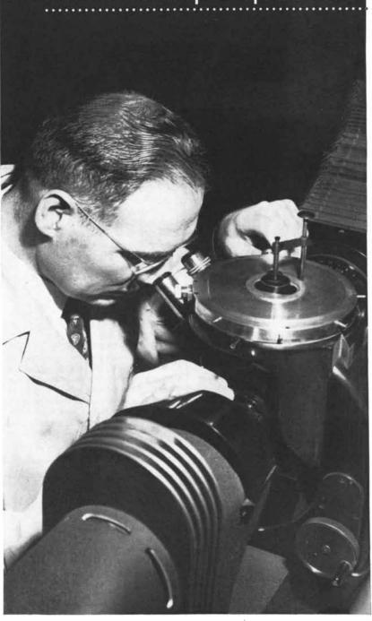
Examining specimen on metallographic microscope at Bell Telephone Laboratories.
