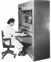
The precision inherent in the Model 21-201 Consolidated-Nier Isotope-Ratio Mass Spectrometer makes possible the use of stable isotopes for tracer techniques in fundamental studies. This instrument is in use in numerous medical, biological, and chemical research laboratories throughout this country and abroad, and has played an important role in recent discoveries and scientific advances.
