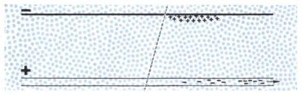
**IMPULSE** moves along wire as electrons are freed of attraction of positive ions. The positive ions are neutralized at the negatively-charged cylinder.
