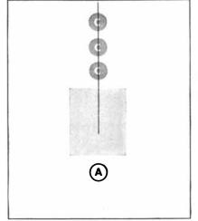
**PENETRATING** cosmic-ray particles are counted to the exclusion of showers of particles by a special "anti-coincidence" arrangement of counters. Penetrating particle passing only through counters labeled C is counted; shower, passing also through counters labeled A, is not.
