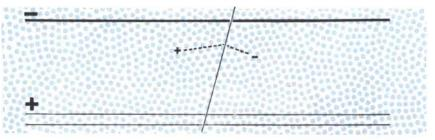
**ELEMENTS** of a counter in a highly schematic cross section are cylinder (*top*) and wire (*bottom*). A ray passing between them mutilates a gas atom.
