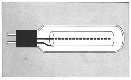
**STANDARD COUNTER TUBE** is basically a positively-charged wire surrounded by a negatively-charged cylinder. These parts are enclosed in a gas-filled glass envelope which may be mounted upon a standard tube base.
