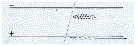
**ION CLOUD** drifts toward the negatively-charged cylinder. Electrons, still held in place by attraction of positive ions, begin to move along the wire.
