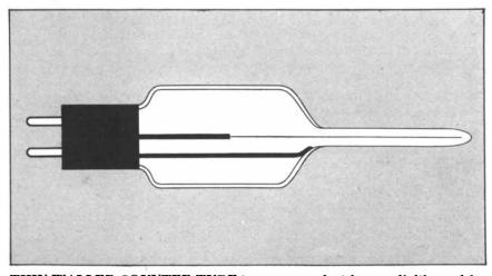
**THIN-WALLED COUNTER TUBE** is constructed with a needlelike end for insertion into radioactive liquids or tumors. Here cylinder is replaced by a thin metal coating that is deposited on the interior of the glass envelope.
