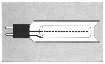
**THIN-WINDOW COUNTER TUBE** has a thin glass window at one end to admit those particles which cannot penetrate the glass envelope of the standard tube. Sometimes the radioactive material is placed within the counter.
