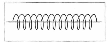
**LONG COIL** may be used to focus beam of electrons. When current passes through the coil, it is surrounded by a magnetic field parallel to its axis. The field exerts no force on electrons moving parallel to the coil's axis, but electrons crossing the magnetic lines of force are turned back toward the axis.
