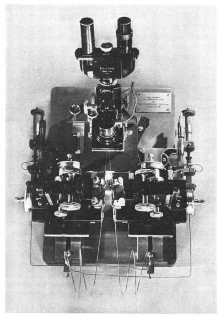
**PRECISION MICROMANIPULATOR** permits the insertion of two micropipettes into cells on the stage of a special inverted microscope. At the upper left and right of the photograph are micrometer-controlled syringes.
