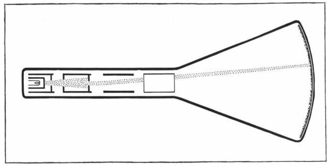
**CATHODE-RAY TUBE** may utilize two sets of plates such as those shown at the bottom of page 34 to move an electron beam in three dimensions. At the left end of the tube is an electron gun. To the right of it is one pair of
