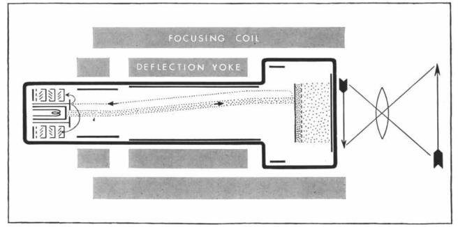
**IMAGE ORTHICON** is a television camera tube. At right end of tube an image is focused on a photoelectric surface. Electrons emitted from the surface in the pattern of the picture are then amplified by secondary
