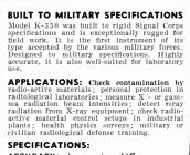
ACCURACY: plus or minus 10% RANGES: 0-5, 0-50, 0-500, 0-5,000, 0-50,000 mr/hr. TEMPERATURE RANGE: minus 10°F. to plus 125°F. POWER SUPPLY: Self-contained batteries. CASE: Immersion proof, grey Hammertone
