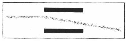
**TWO PARALLEL PLATES** may be used to deflect an electron beam. If one of the plates is made positive with respect to the other, the electron beam is bent toward the former. The charge on the two plates may rapidly be altered to move the electron beam (see the tube drawing at the top of page 36).
