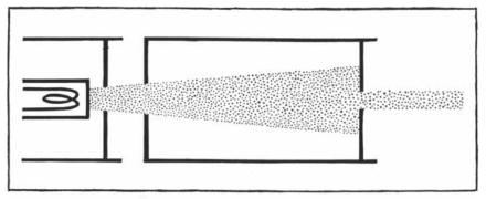
**ELECTRON GUN** is the fundamental means of producing a beam of electrons. In this schematic drawing the cathode is the electron-emitting surface at the far left. The electrons travel through a hole in the grid and through another hole in the anode. The third hole defines the beam more sharply.
