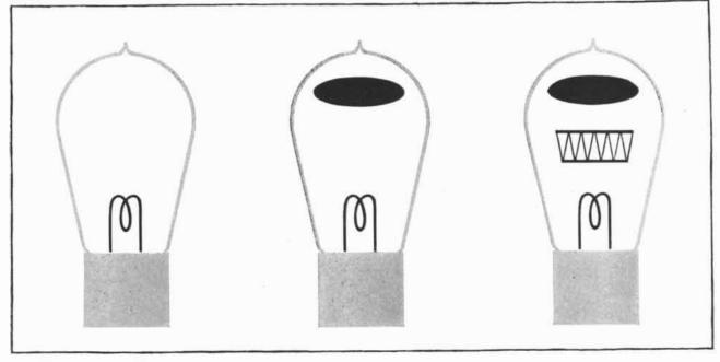
**THREE BASIC ELEMENTS** of electronic tubes are cathode, anode and grid. The cathode is a negatively-charged electrode which emits electrons. The anode is a positively-charged electrode which attracts electrons.
