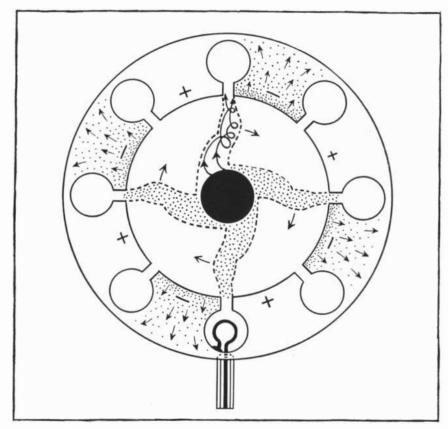
**MAGNETRON** has resonant cavities in a metal ring. Around the ring is established a magnetic field whose lines of force are perpendicular to this page. The electrons describe curved paths between cathode (*center*) and ring, and give up their energy by interacting with electric field of cavities.
