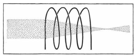
**SHORTER COIL** may be used as a magnetic lens to focus electrons. Near the center of the coil the magnetic lines of force are parallel to its axis. Toward the ends of the coil, however, the lines of force bend away from the axis. An electron entering the coil away from the axis is thus forced toward it.
