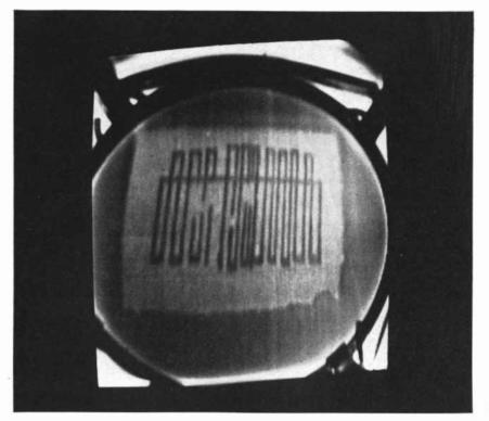
**MEMORY TUBE**, developed by Andrew V. Haeff of the Naval Research Laboratory, is a memory device for electronic computing machines. The tube can remember either numbers or pictures for hours or days, and reproduce them on demand. On the face of tube is a meaningless test pattern.
