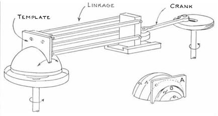
This linkage will automatically produce a paraboloid
