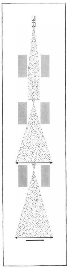
**ELECTRON MICROSCOPE** utilizes several focusing coils to manipulate electron beam and produce vastly enlarged image of specimen.
