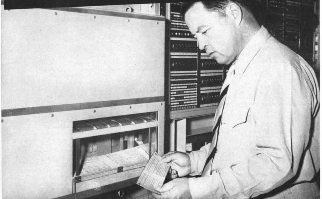
Studying punched card record of dial system operation. Each card (top) can report 1080 items
