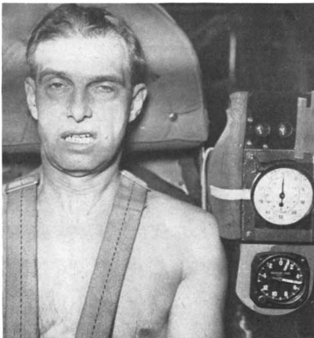
high acceleration. The effects of acceleration are recreated in these photographs, which show a human subject being whirled in the great centrifuge of the Air Force Air Materiel Command at the Wright-Patterson
