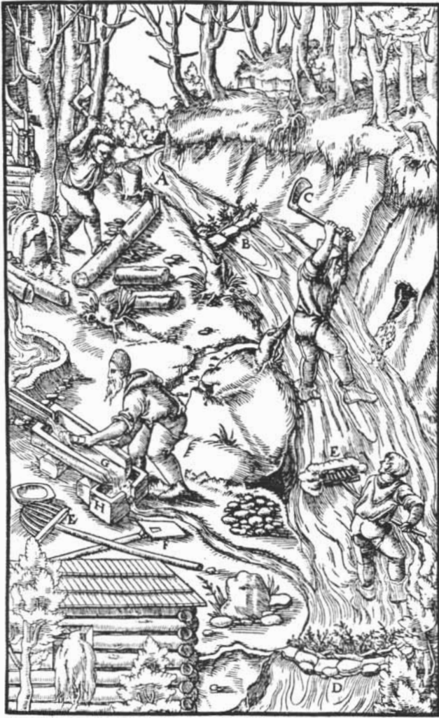
TIN ore was washed by diverting a stream into a ditch near the deposit. The miners then threw the ore into the ditch to wash away everything but stones bearing tin.
