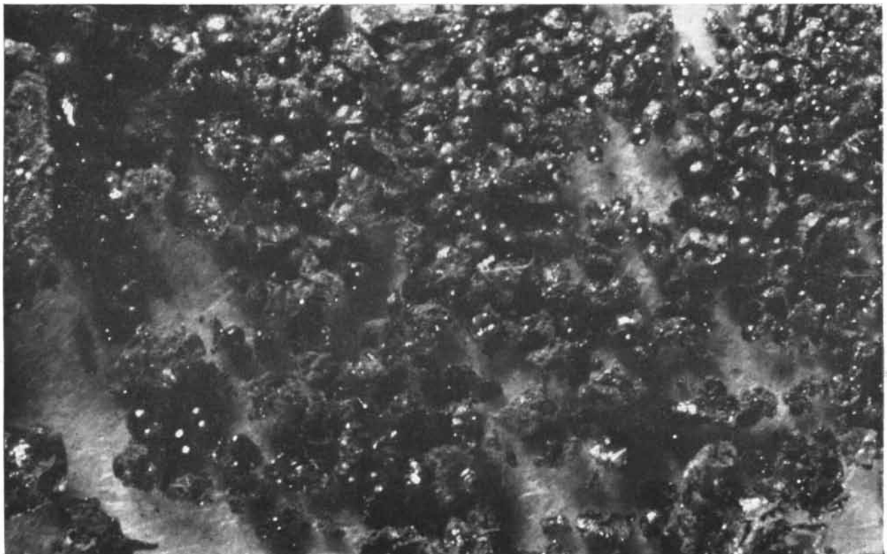
MELTED GLOBULES of steel appear in the dust after the saw has been running a short time; the saw appar-
