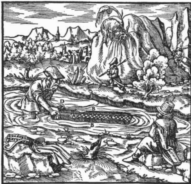
GOLD was sometimes washed by miners standing in streams. When the ore was placed in the frame, the gold settled near the handles and the waste washed away.
