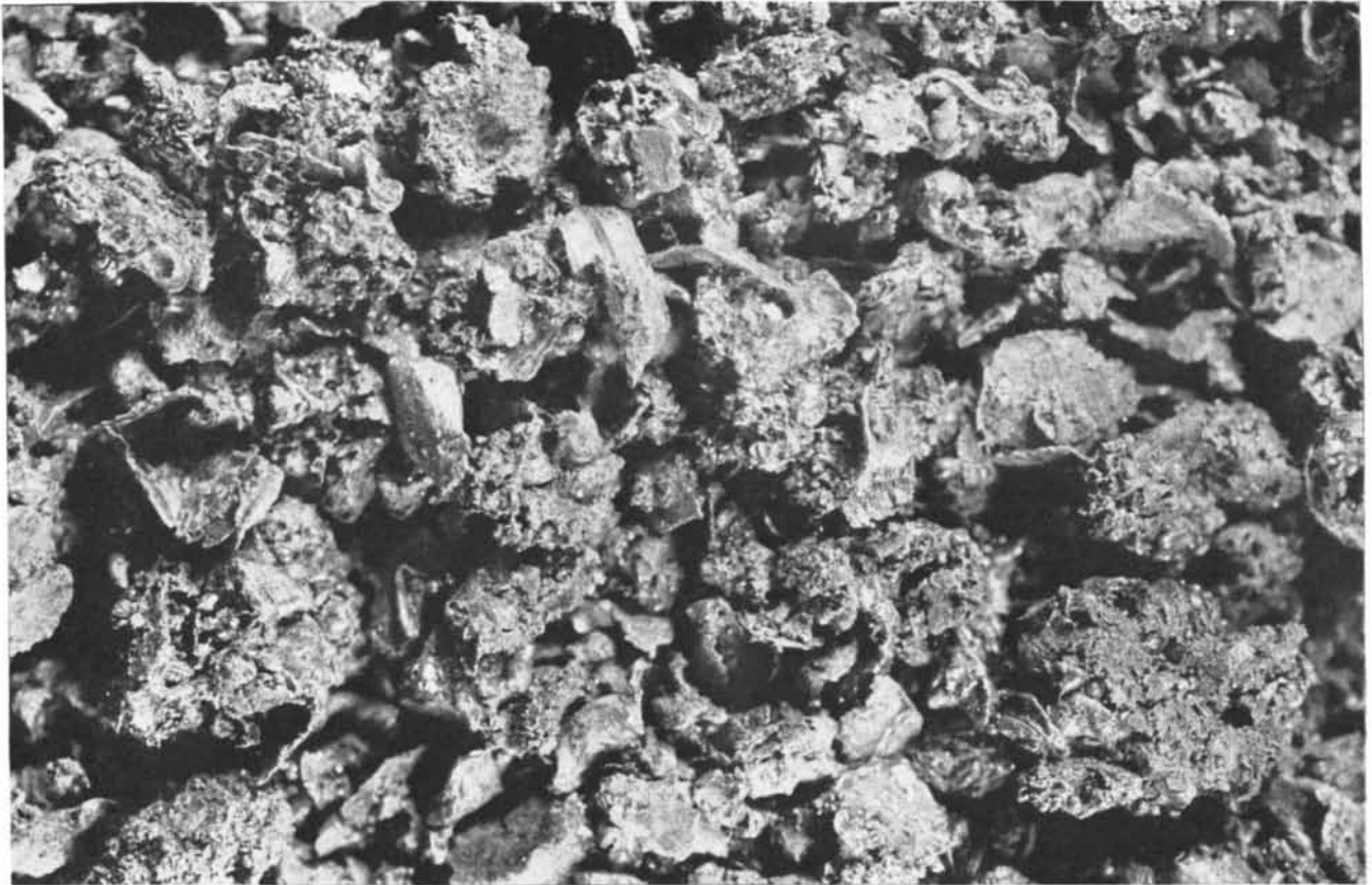
STEEL SAWDUST is from a circular friction saw beginning to cut through a piece of steel. Such a saw is
