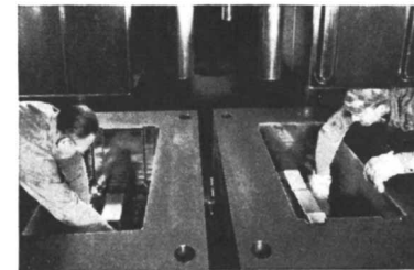
Preparing for 40 lb. plastic charge. This is Crucible's 9300-lb. CSM2 forging.
