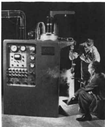
Transferring liquid helium to external dewar. A built-in test chamber also allows tests within the cryostat controlled temperatures down to -271^{\circ}\text{C} (within 2 degrees of absolute zero).
