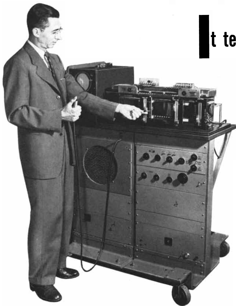
The machine at the left is saying "Ah!" It's the new electrical vocal system developed at Bell Laboratories. Top sketch shows human vocal system also saying "Ah!" The electrical model is sketched below it. Energy source at bottom of "tract" can emit a buzz sound, like vocal cord tone, or the hiss sound of a whisper.
