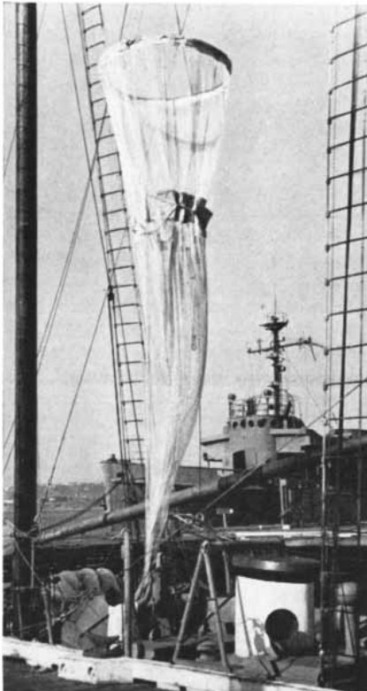
SIX-FOOT NET was also used to catch plankton. It is rigged for opening and closing while in the water.
