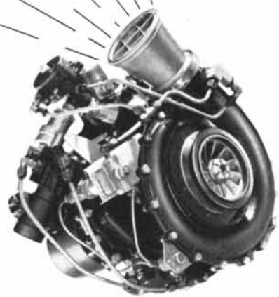
The new AiResearch supercharger (cabin pressurization compressor) has the highest efficiency rating ever achieved in equipment of this kind.
