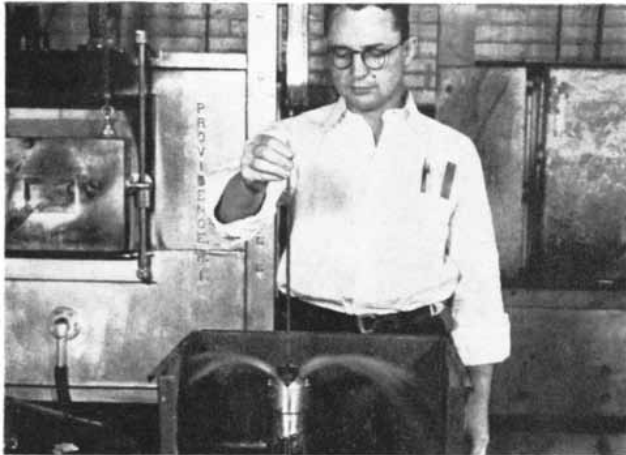
A P-V specimen is quenched in a standard fixture. This is part of a special procedure for determining the hardenability of high quality shallow hardening tool steels. After this operation, the V-shape specimen is cut longitudinally and tested for hardness on the Superficial Rockwell machine.
