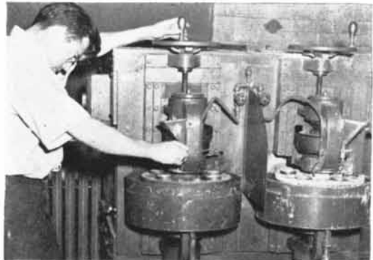
Automatic polishing of test samples for use in examinations for decarburization, microstructure, inclusions.
