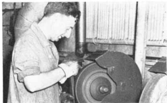
This is part of Crucible's mirror finishing equipment which is patterned after that of the cutlery manufacturers to whom Crucible furnishes mirror finish stainless steel. The polishing operation is designed to simulate that performed by the manufacturer in the production of high grade cutlery.
