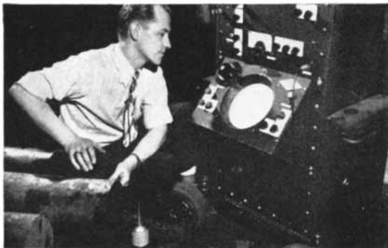
Checking structure of large bars ultrasonically for internal defects.
