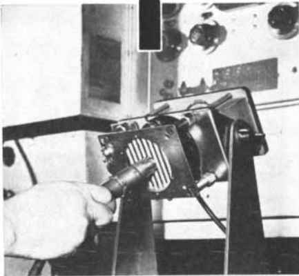
At Bell Laboratories a scientist employs a condenser microphone to check the sound level from another type of artificial mouth, used in transmitter research.
