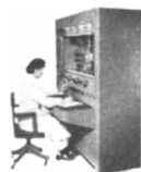
Model 21-201 Isotope-Ratio Mass Spectrometer - specifically for measuring ratios of stable isotopes in gases.
