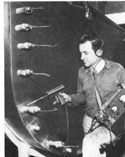
Locating minute leaks in 1000-gallon milk tank with G-E Leak Detector.
