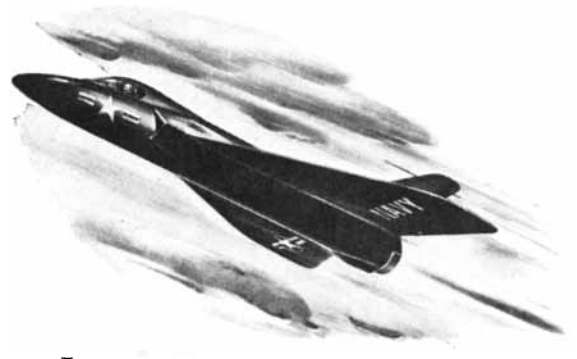
Jet... Designed for intercepting high-flying supersonic enemy planes, the F4D Skyray is an advanced-type bat-wing jet, developed by Douglas for the U. S. Navy.
