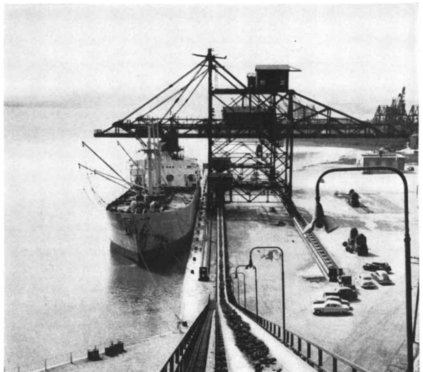
ORE CARRIER of the Republic Steel Corporation which has brought a cargo from the Bomi Hills of Liberia is unloaded by conveyor at Baltimore.
