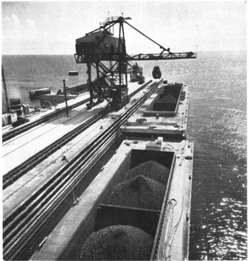
BARGES carrying iron ore from Bethlehem Steel's Venezuela workings are unloaded at Puerto de Hierro. The ore is moved to ocean-going carriers.
