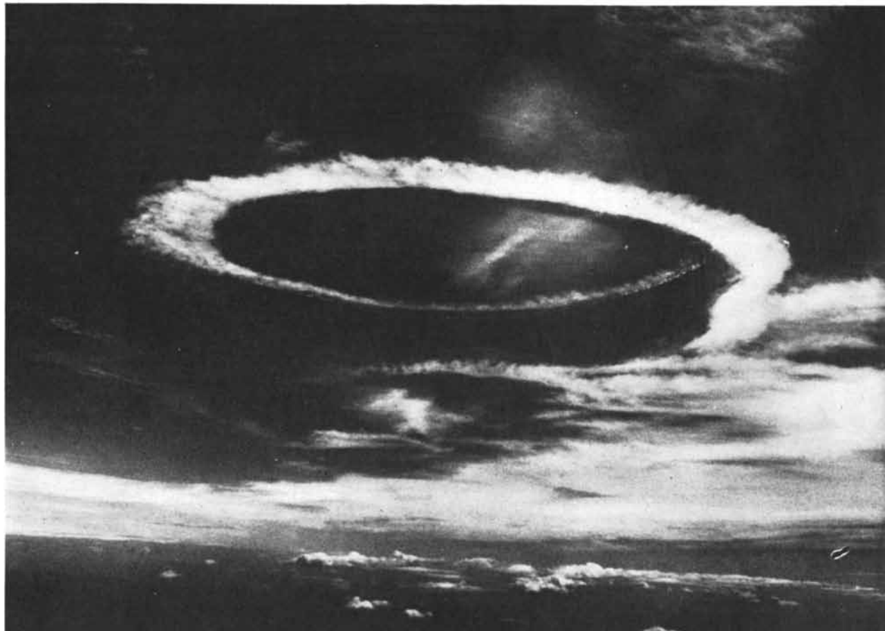
SILVER-IODIDE SEEDING made this circular pattern in relatively clear air. The experimental aircraft flew in a circle five miles in diameter at an altitude of 26,000 feet while it released a trail of silver-iodide smoke.
