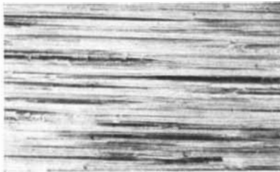
Faxfilm of steel surface with ground finish. Faxfilm is excellent for checking best speeds, feeds, and lubrication for machining.
