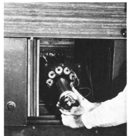
GEIGER COUNTER finally measures the amount of radioactivity in the carbon prepared from the sample.
