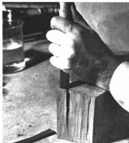
SAMPLE IS SPLIT from a block of wood being dated in Geochronometric Laboratory of Yale University.
