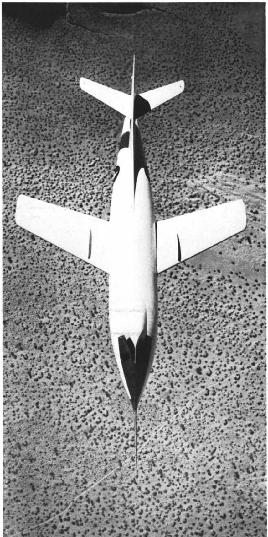
DOUGLAS SKYROCKET , a rocket-powered aircraft, has been reported to have reached an altitude of 15 miles. It was borne aloft from Edwards Air Force Base near Muroc, Calif., by a B-29 bomber and launched in the air.
