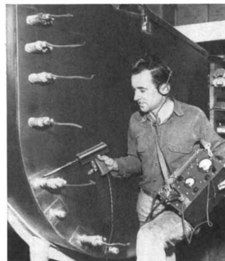
Locating minute leaks in 1000-gallon milk tank with G-E Leak Detector.
