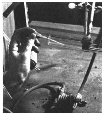
SAMPLE IS PLACED in a heating tube at the beginning of the process of converting it into carbon dioxide.
