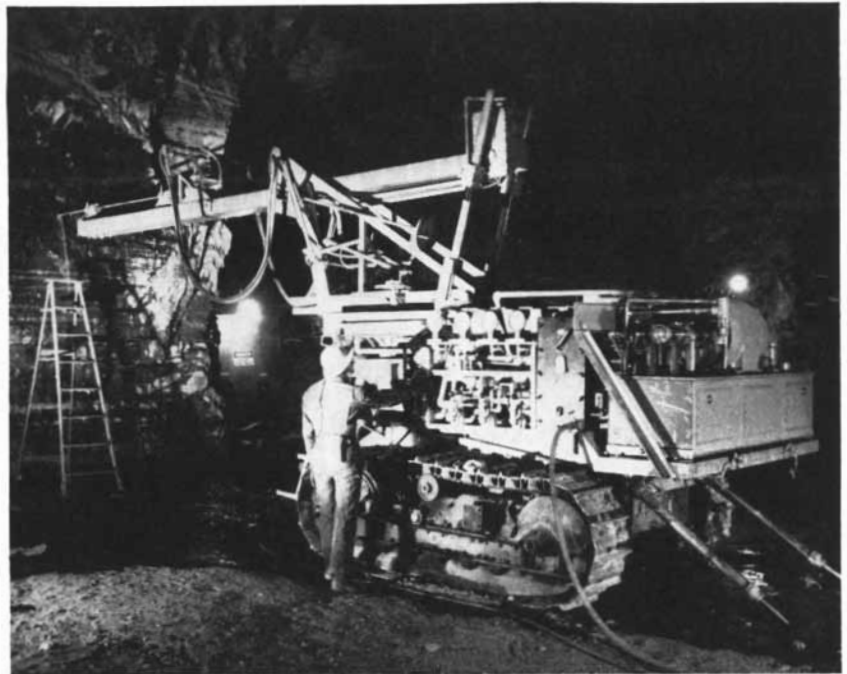
EXPERIMENTAL DRILL is used to make holes for blasting in the mine of the Demonstration Plant. One blast can loosen some 1,700 tons of shale.
