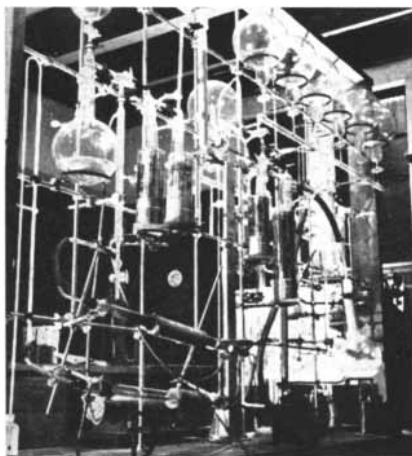
CARBON DIOXIDE from the sample is dried by freezing ( center ) and stored in glass bottles ( upper right ).
