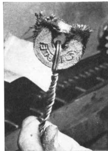
Magnet shows metal chips removed from shaver heads by ultrasonics.
