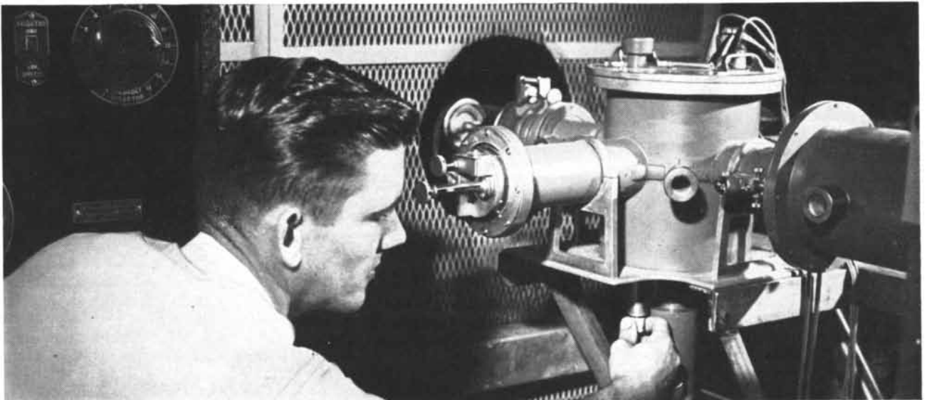
3 A Bell scientist adjusts electron diffraction camera. Electrons are projected on the specimen at glancing angles. They rebound in patterns which tell the arrangement of the atoms . . . help show how telephone materials can be improved.
