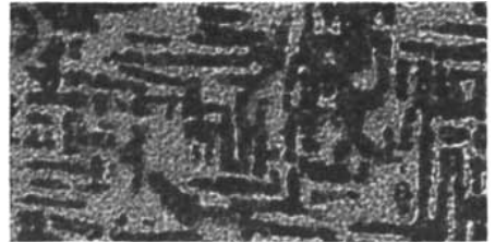
1 Electron micrograph of an alloy of aluminum, nickel, cobalt and iron. Magnification 20,000 diameters.
