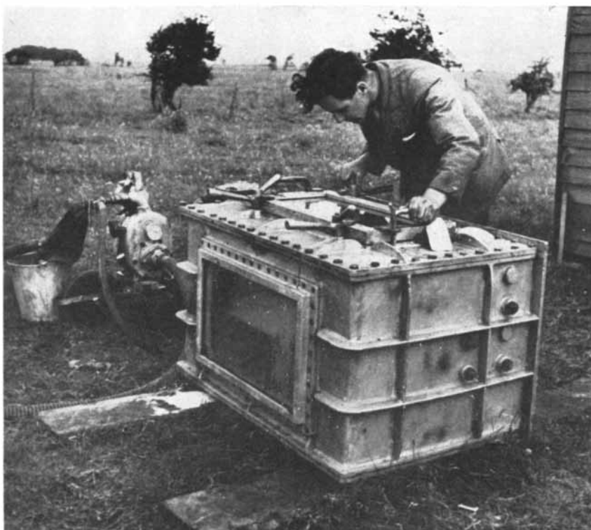
VACUUM CHAMBER was brought to the Star Carr site by the archaeological party to impregnate fragile animal remains with polyvinyl acetate.
