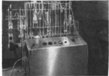
Vacuum Fusion Gas Analyzer. Analyzes metals and alloys, including titanium, for combined or dissolved oxygen, nitrogen, and hydrogen.
