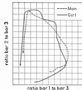
The word "five." Graph shows ratio of frequency of spectrogram bars. The solid line is for a girl and the dotted line is for a man. Note the similar patterns despite pitch differences. Human hearing extracts the speech sounds from this sort of pattern in the identification of words. Scientists aim at machines that can do the same.
