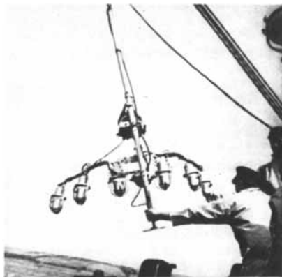
CAMERA for underwater photography is swung overboard. It is mounted above the semicircle of lamps.
