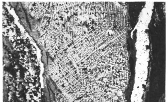
CROSS SECTION OF BRONZE from China shows corroded metal in center and cuprite at left. The bright streaks at left and right are redeposited copper.
