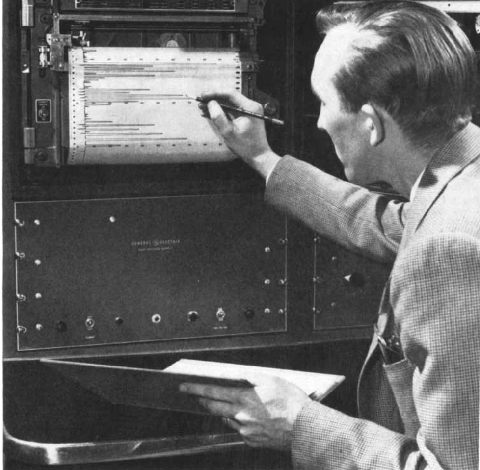
Operator observes cracking pattern of natural gas sample with G-E Mass Spectrometer.
