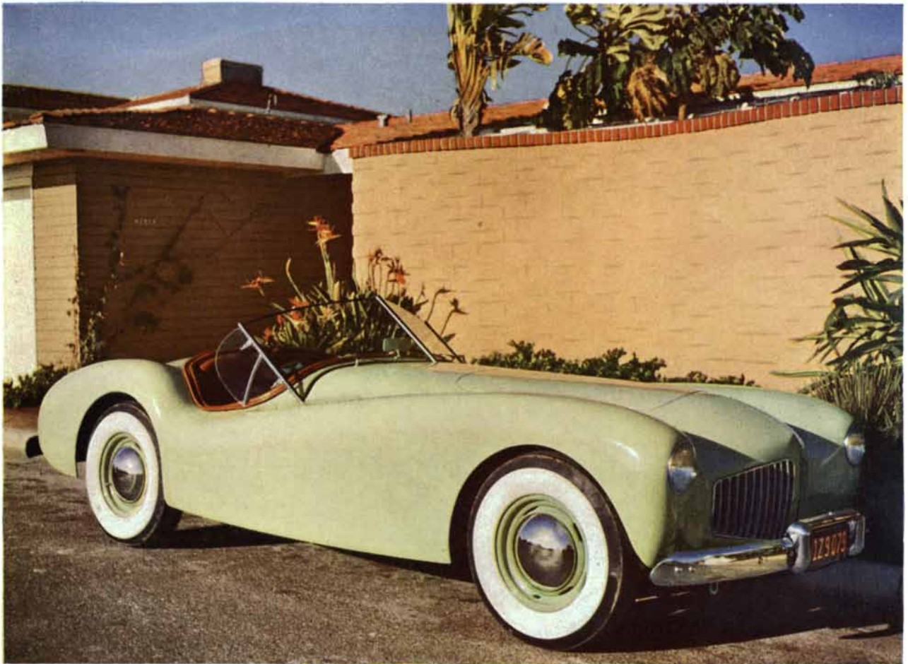
Experimental model made of Vibrin polyester resins and glass fibers by Glasspar Company, Costa Mesa, California
