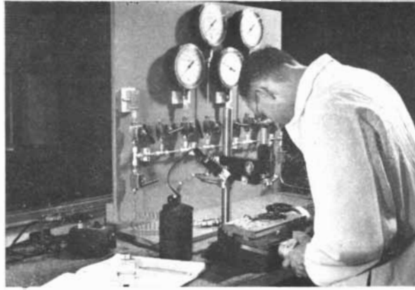
HONEYWELL NUCLEAR ENGINEERING LABORATORY. Research in the measurement of physical characteristics of Uranium-238 is facilitated by the machining of a clean surface.
