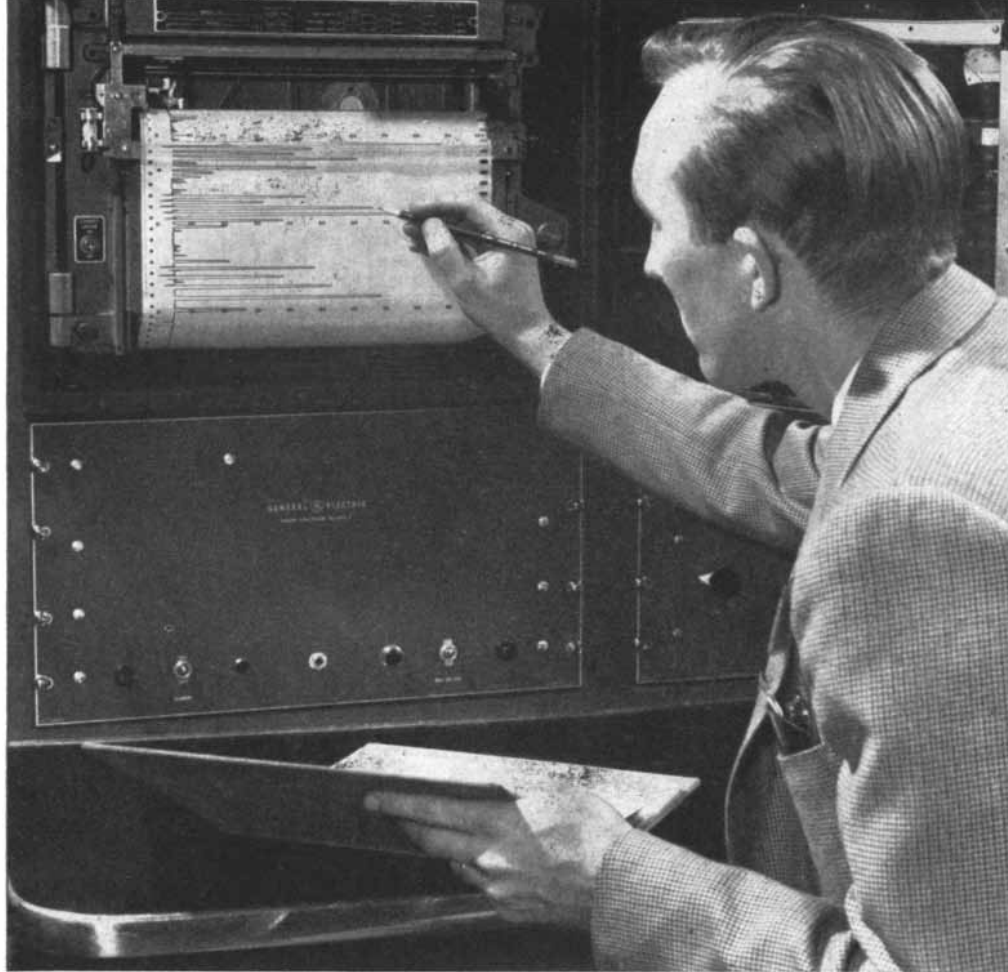
Operator observes cracking pattern of natural gas sample with G-E Mass Spectrometer.
