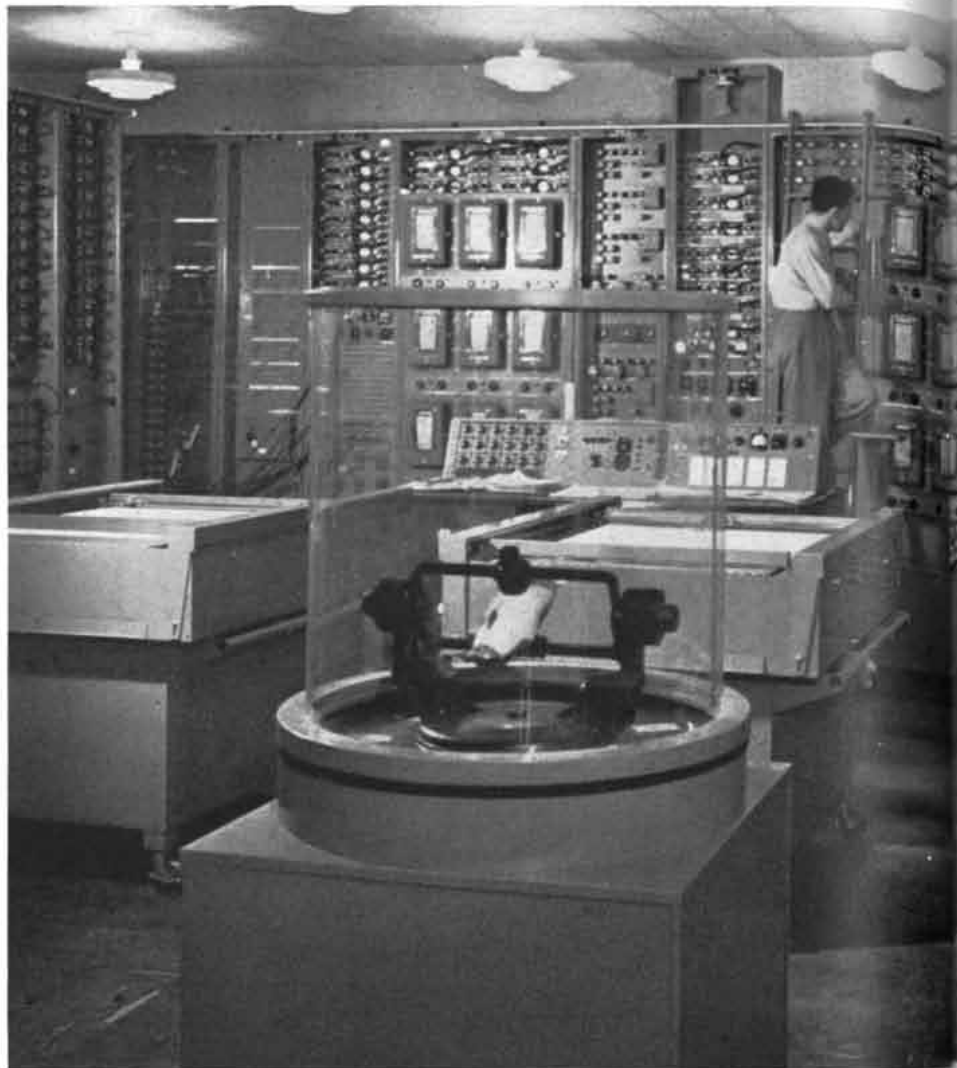
LARGE ANALOGUE COMPUTER is exemplified by the machine of Project Typhoon, built by the Radio Corporation of America to simulate the
