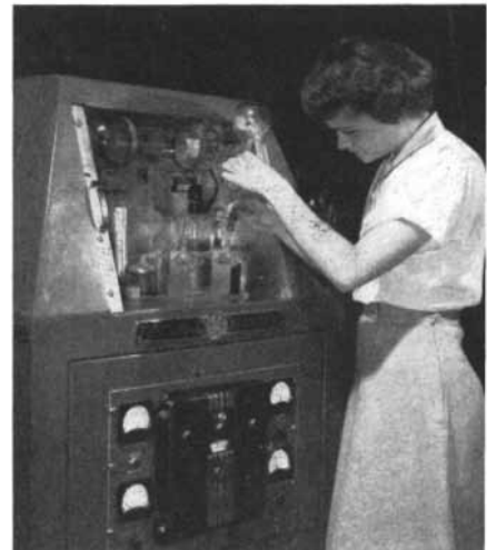
Convenient sample system facilitates introduction of unknown gas mixture.
