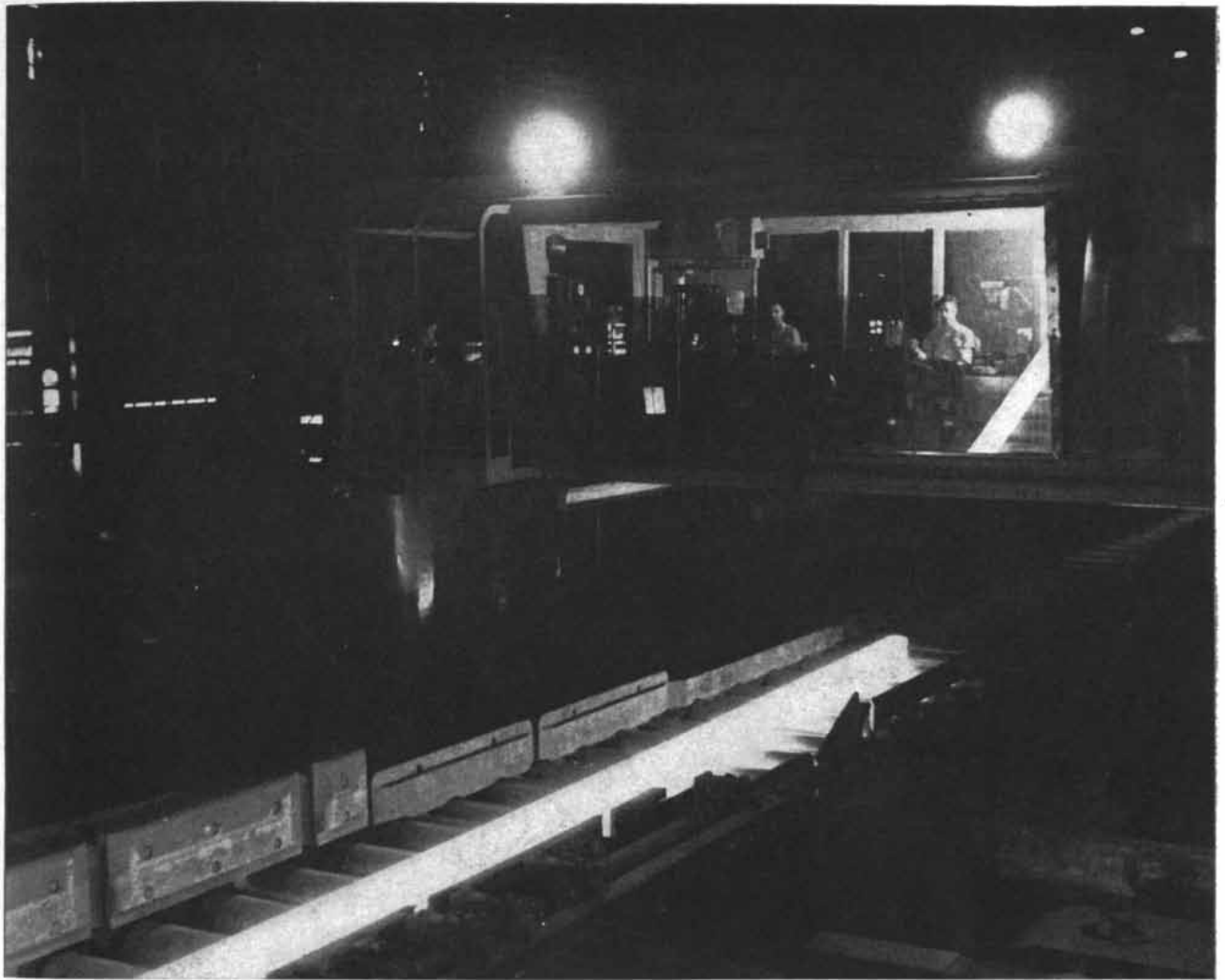
BLOOMING MILL in the Lorain Works of the National Tube Division is operated by a direct-current servo-
