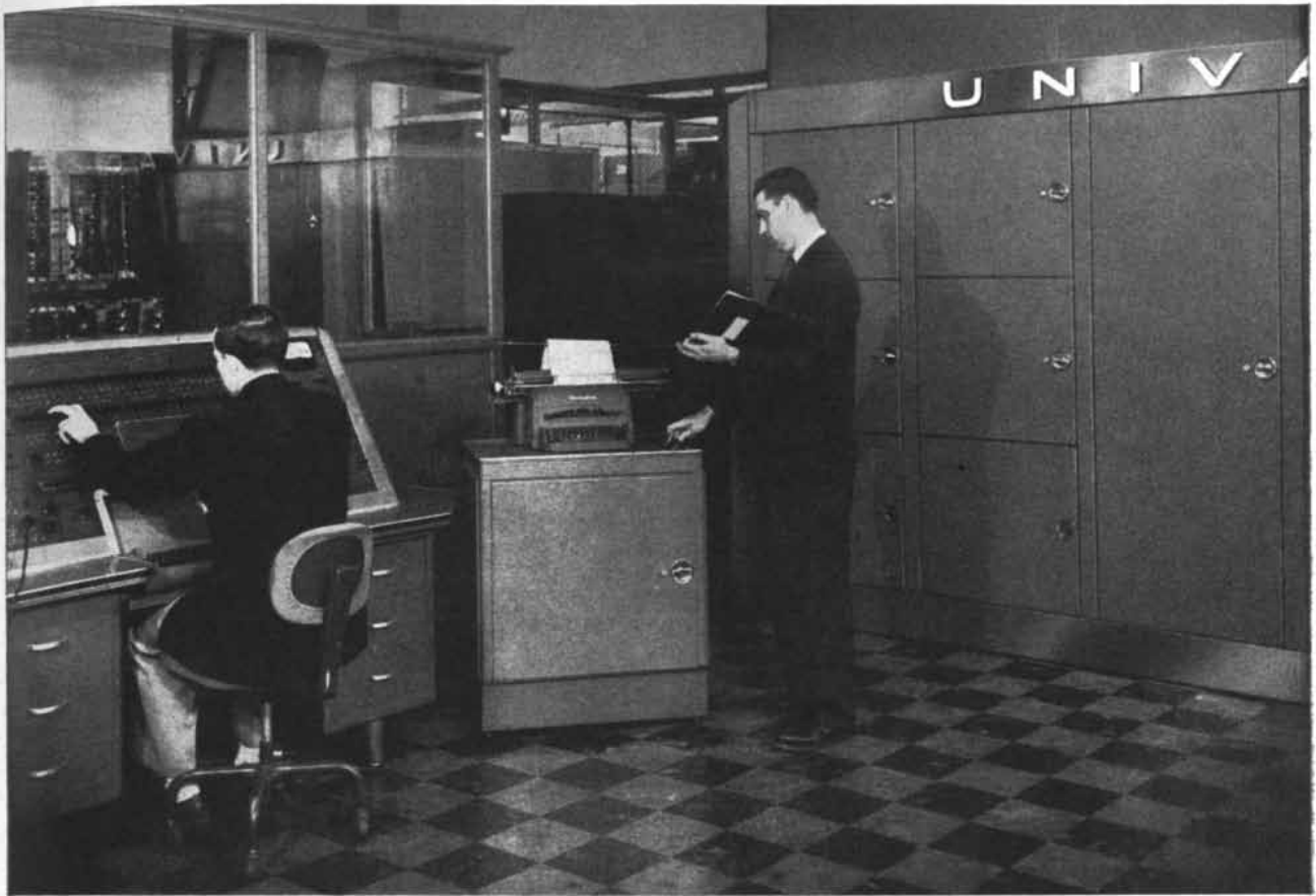
The Univac Fac-tronic System processes both numeric and alphabetic data from metallic tape without special coding... delivers results in typewritten form ready for immediate use.
