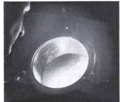
The exceptional heat resistance of sight glasses like this permits you to watch reactions taking place in blazing hot furnaces.
