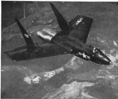
Flight of the Chance Vought Cutlass, seventh in a line of outstanding fighters and "potentially capable" of flying faster than any other service type jet aircraft in production, land or carrier-based. Substantial surface areas of the Cutlass are constructed of painted Alodized aluminum.
