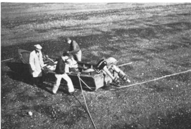
SKIFF from which the cardiogram was made was 20 feet long. The electrocardiographs were mounted in bottom.
