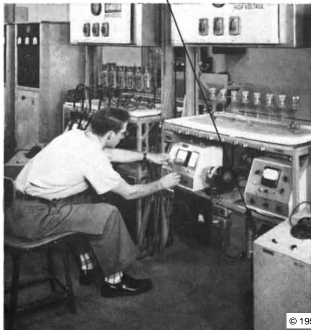
Diffusion Pumps to produce high vacuum at rates up to 50 litres per second from 10^{-8} mm to 10^{-6} mm range against forepressure as high as .300 mm.
