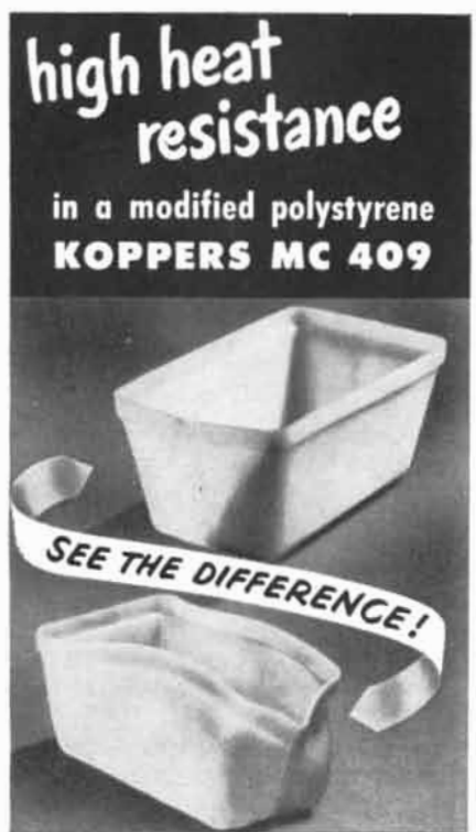
The boxes in these unretouched photographs were molded under the same conditions and exposed to a temperature of 212°F. The box on top, made from Koppers MC 409, showed little or no distortion after 30 minutes at this temperature. The box underneath, made from a widely used commercial modified polystyrene, showed major distortion within 10 minutes.
