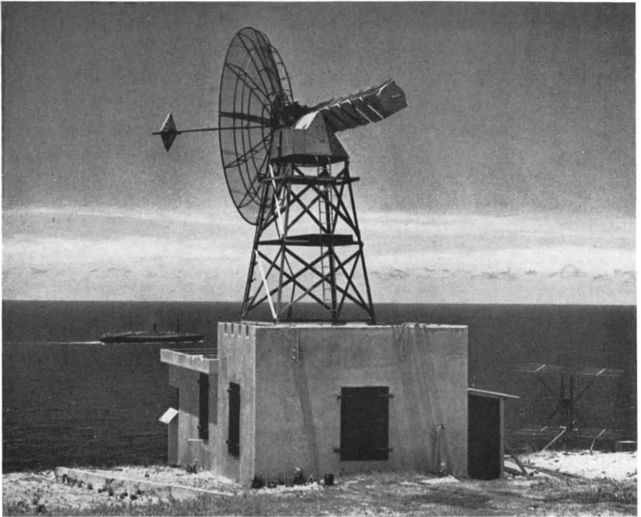
AUSTRALIAN RADIO TELESCOPE overlooks the sea near Sydney. It is part of an interferometer that receives radio waves directly from a source in space and waves from the same source that are reflected from the water.
