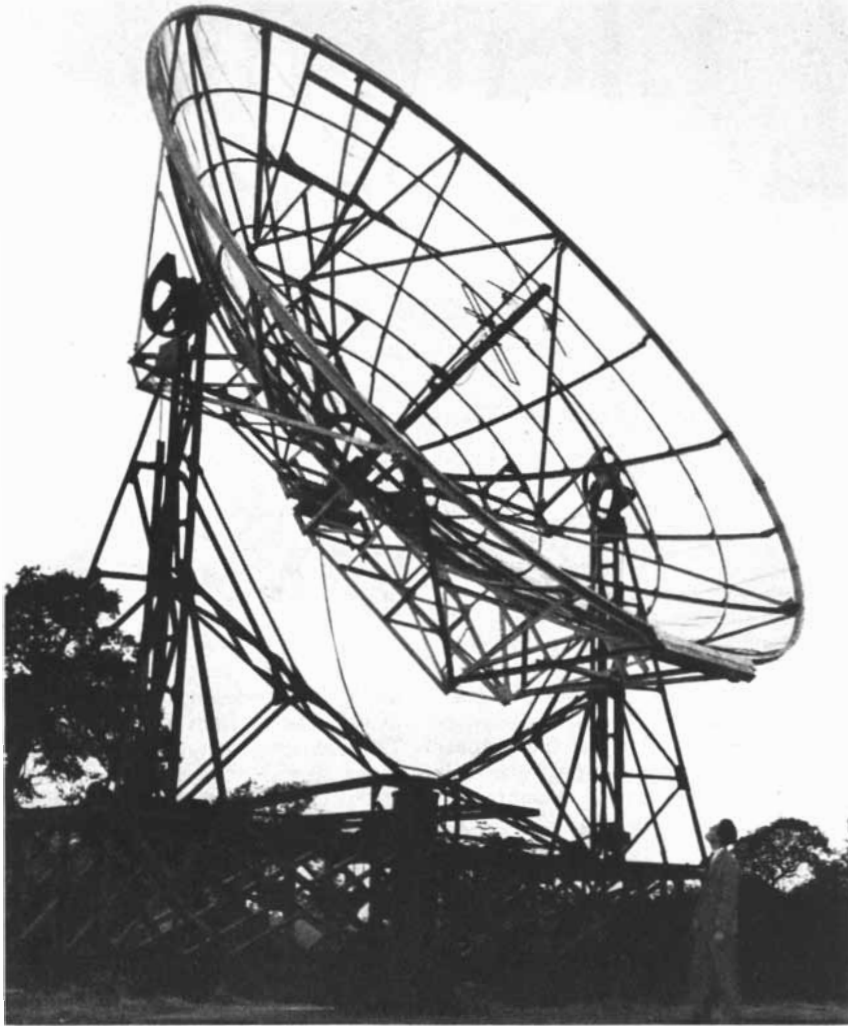
ENGLISH RADIO TELESCOPE has a diameter of 30 feet. It has the same general design as that of the 250-foot telescope now being built.
