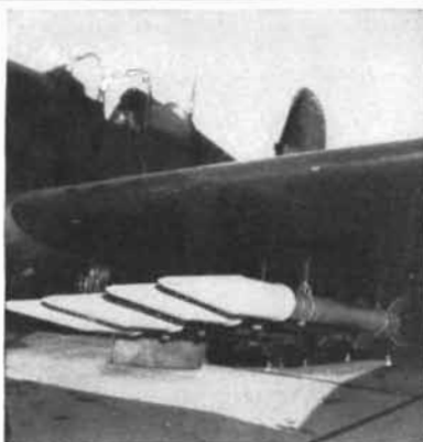
Official Dept. of Defense Photograph An F4U Corsair with the Navy's new aircraft anti-tank rocket, the "RAM". A Grade I zinc phosphate finish (JAN-C-490) protects the entire external surface of this rocket and provides a durable bond for the specification paint finish.
