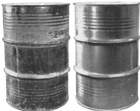
ORDINARY PAINTED DRUM after a year of exposure to weather is badly rusted. Rust was very apparent after only one week.
