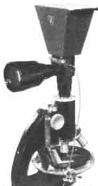
2 1/4" x 3 1/4" camera on B&L Model E Research Microscope
