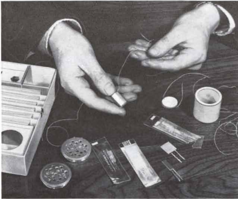
Kit of piezo-electric materials includes: 2 crystal bender Bimorphs®; 2 crystal twister Bimorphs (oblong shape); 2 crystal twister Bimorphs (square shape); 1 Ceramic "B" disc; 1 Ceramic "B" tube; 1 Ceramic "B" hexagon; 2 microphone cartridges of the hearing-aid type; Instruction sheet.
