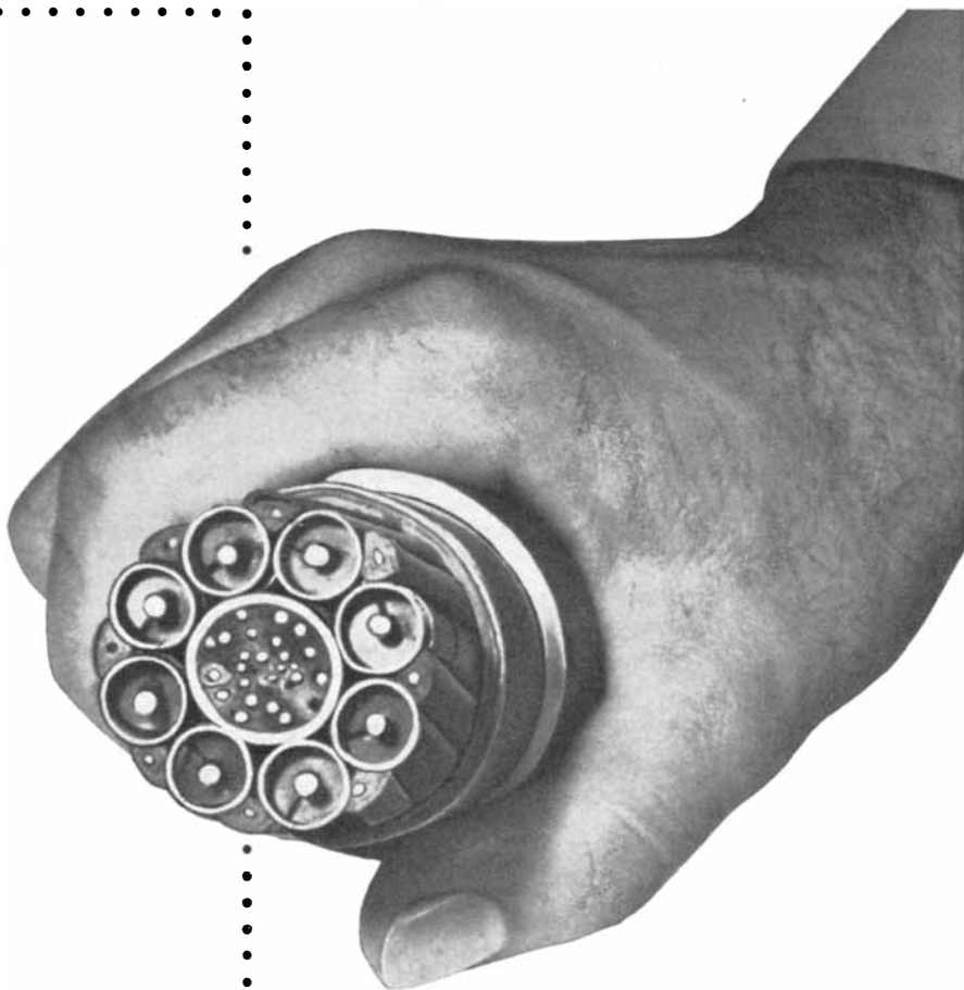
Cross-section of coaxial cable. To triple capacity, Bell Laboratories and Western Electric engineers had to make 1000 amplifiers work perfectly in tandem . . . feed repeater power along the same cable that carries messages . . . put signals on and off the line at numerous cities along the route without distortion.
