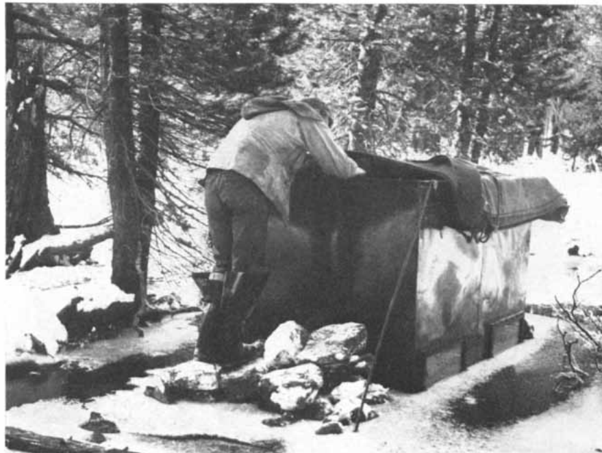
OBSERVATION TANK is sunk in Sagehen Creek so the behavior of trout may be observed. Here the windows of the tank are visible at low water.
