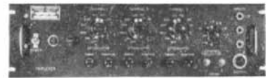
TRIPLEXER —when coupled to a DC amplifier permits the recording of three events in one channel.
