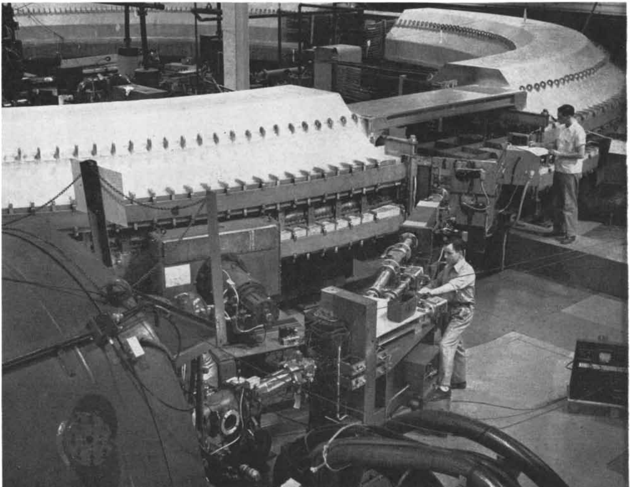
VAN DE GRAAFF GENERATOR (large tank at lower left) injects protons into the Cosmotron with an energy
