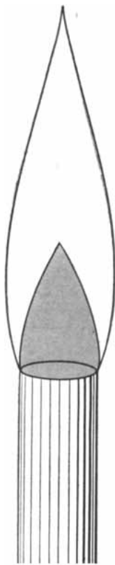
ETHYLENE-AIR FLAME shows two-cone form of simple gas flames. Inner one is bright, outer pale blue.
