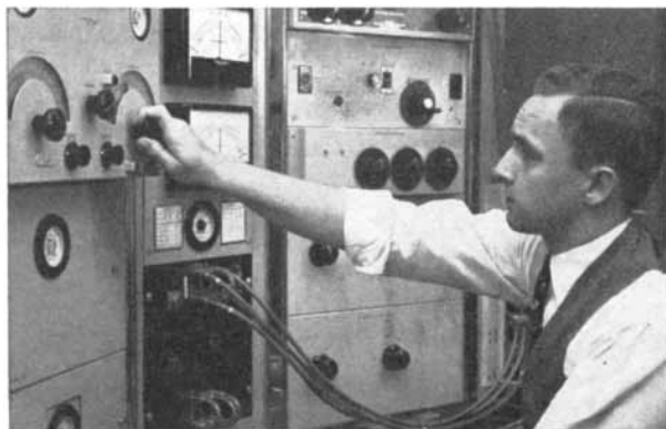
Laboratories engineer tests new triple-duty coaxial system. It marks the first time that telephone conversations and television can travel through the same pipes at the same time. With a wider frequency band being transmitted, big problem was to eliminate interference between the two types of signals.
