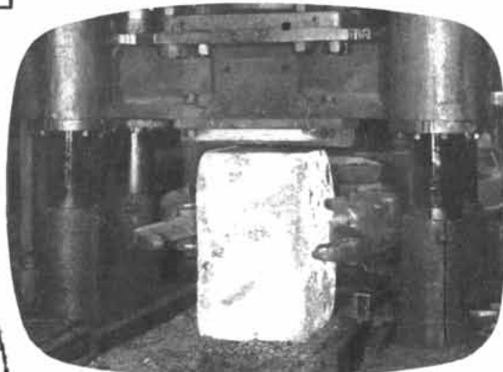
Crucible Plastic CSM2 Mold Steel in final forging stage.
