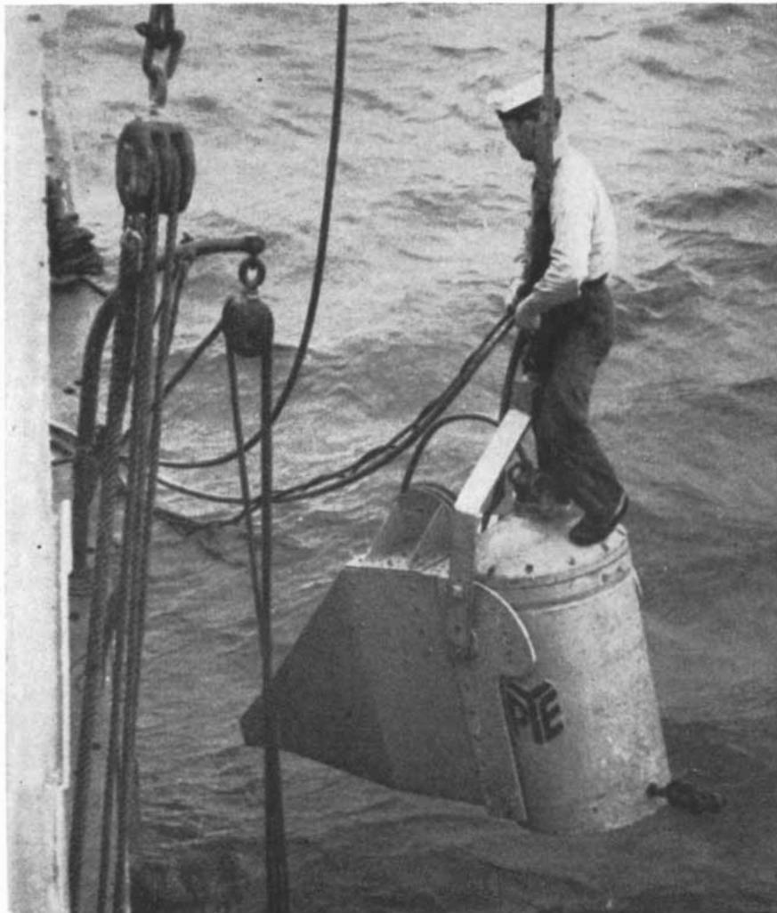
TELEVISION CAMERA protected by a heavy casing is suspended from the Reclaim , the British Navy's deep-sea diving and diving-research vessel.
