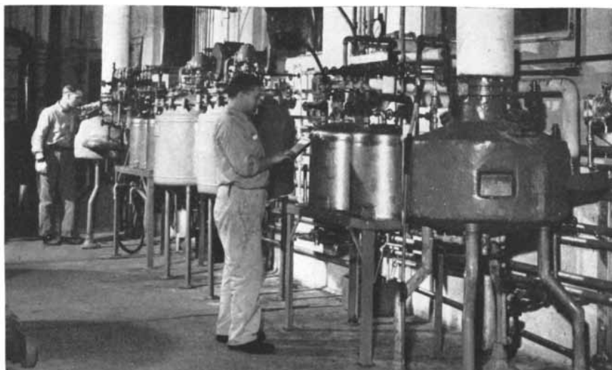
VACUUM STILLS fractionate fruit and flower extracts used in perfumes, which are obtained by modern steam or solvent extraction processes.
