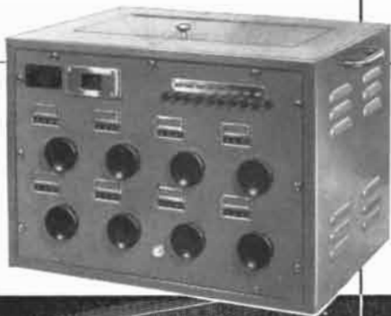
The Simultaneous Equation Solver, an integral part of Baird Associates, Inc. new spectograph, is a simplified analog computer that resolves the machine's complex data output.
