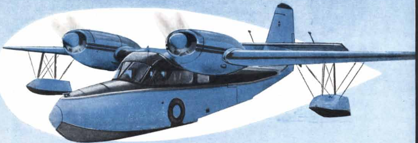
Grumman Widgeon Conversion. Amphibious flying "office" featuring 260-h.p. air-cooled, geared engines by Lycoming.
