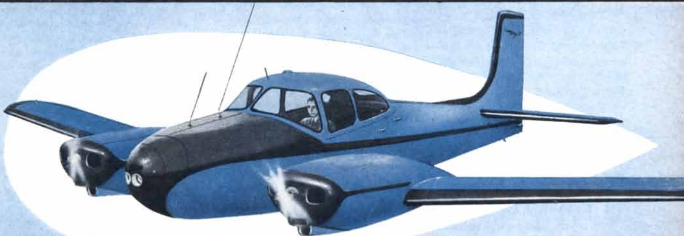
Riley Twin Navion Conversion. 4-place executive plane powered by two 150-h.p. air-cooled Lycoming engines.
