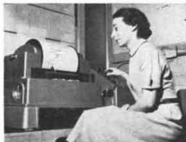
Complete spectrum can be run in 8 minutes on Model 21; material is recoverable.
