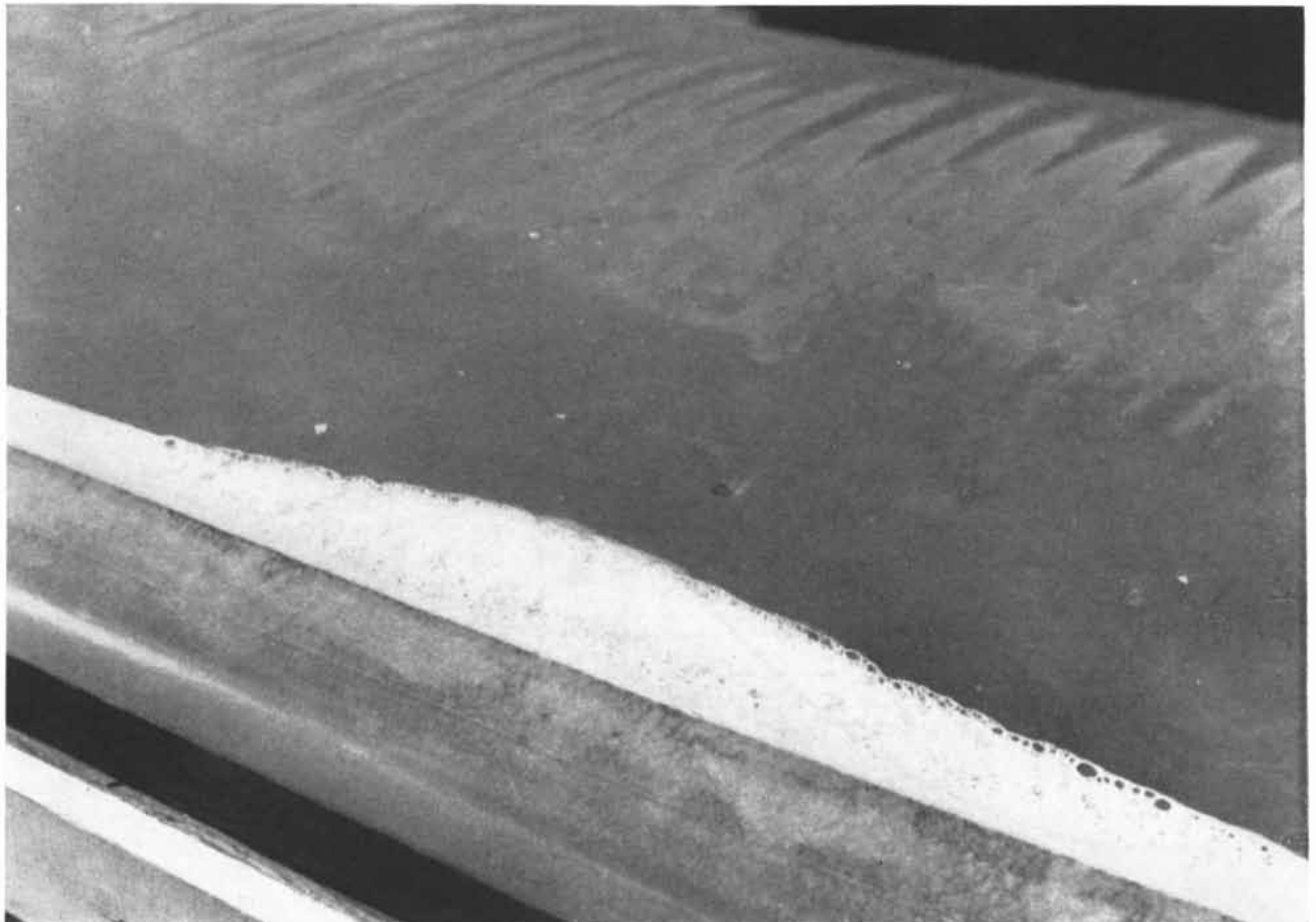
POLYETHYLENE TUBE in pilot plant is pictured in close-up. The space above the foaming culture is filled with a circulating
