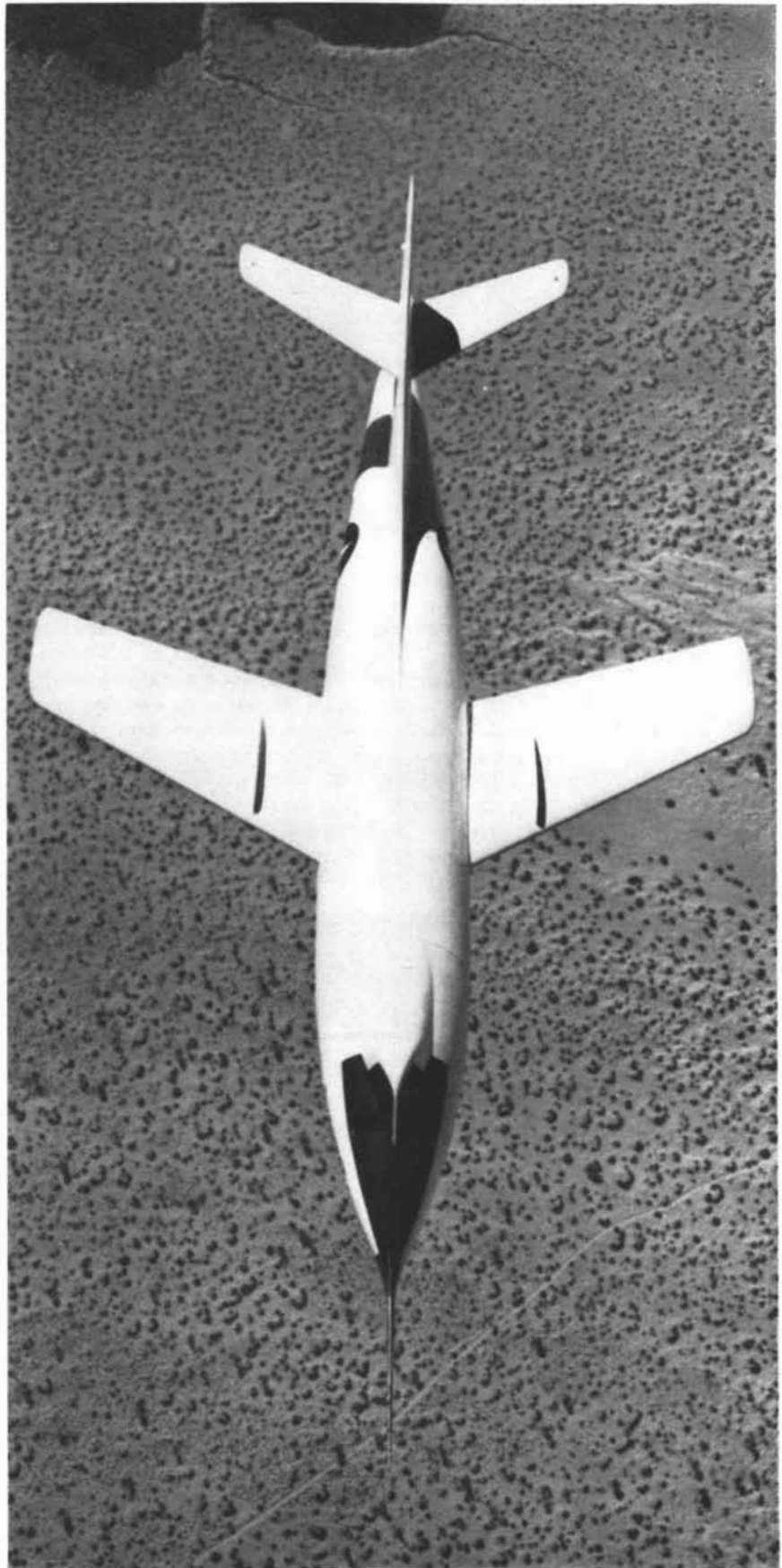
SKYROCKET holds announced speed and altitude records in N.A.C.A. research program. Note vertical fins, "fences," on wings, added to cure plane's tendency to roll at high speeds.
