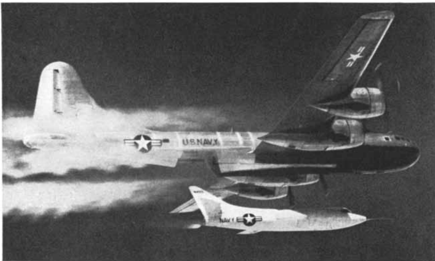
SKY LAUNCHING permits maximum utilization of Skyrocket's brief flight range in research flying. With fuel exhausted the airplane can come down at reasonable landing speed.
