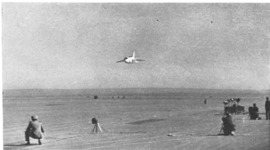
TEST FLIGHT of Skyrocket at low altitude over Muroc desert is monitored by battery of instruments (right). Airplane is formally designated D-558 II, and was built by Douglas.
