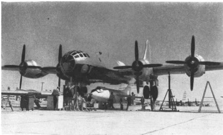
MOTHER SHIP , a modified B-29 bomber, is lifted high on jacks and the Skyrocket is wheeled underneath for pickup preparatory to a high altitude launching on a research flight.
