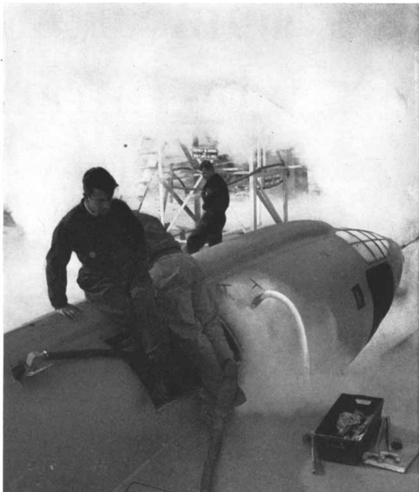
FOG OF LIQUID OXYGEN surrounds Bell X-1 during fueling. Oxidizers needed in rocket airplanes, added to explosive fuels, multiply the accustomed ground hazards of aviation.
