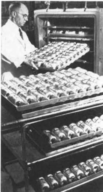
Operator loads shell-frozen human blood plasma into one of the Stokes drying chambers of the lyophilizing plant at the Sharp & Dohme, Inc. biological laboratories, Glenolden, Pennsylvania.
