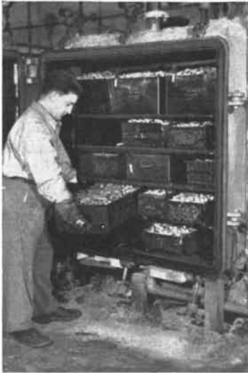
Operator removes boxes of tubular paper capacitors from Stokes Vacuum Impregnator at Pyramid Electric Co., North Bergen, N. J. Capacitors have been impregnated with mineral oil to improve stability and lengthen service life.
