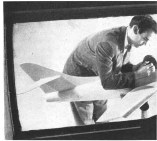
WIND TUNNEL MODEL of Skyrocket is fitted with "slats" on leading edge of wing.
