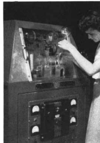
Convenient sample system facilitates introduction of unknown gas mixture.
