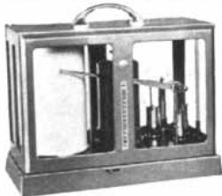
MICROBAROGRAPH A key meteorological instrument. Records atmospheric pressure to within 0.01 inch mercury. Record chart expanded 2\frac{1}{2} times for greater visibility.
