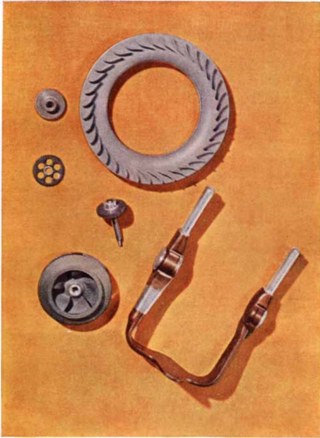
FILE HARD COATINGS . . . New ways to apply an extremely hard, thick anodic coating on aluminum have been developed by Alcoa's finishing labs. Of controlled thickness and density, these coatings offer a high degree of resistance to wear and abrasion.
