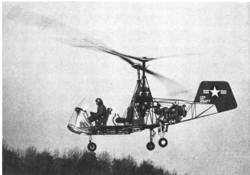
SMALL GAS TURBINE has been developed by the Boeing Airplane Company. It has been installed experimentally in trucks and boats. Here it appears in the back of a helicopter.
