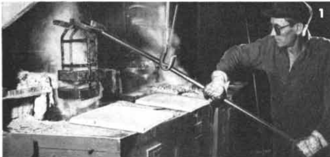
HARDENING — Small batches of REX High Speed Tool Bits are hardened in modern salt bath furnaces. The bits are then quenched in either salt or oil.
