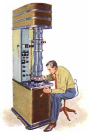
Electron microscope capable of magnification up to 100,000 diameters.
