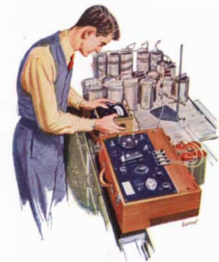
Electrolytic solution potential test equipment for studying corrosion problems.
