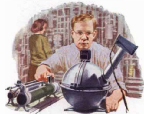
Measuring the light reflectivity of aluminum sheet.
