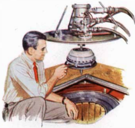
Whirlpit for testing performance of rotating parts up to 80,000 rpm.
