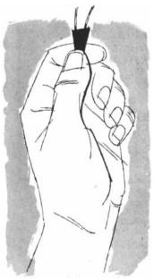
Tiny crystal element, typical of crystals supplied by Brush to phonograph and pickup manufacturers. The crystal pickup translates the grooves on a phonograph record inlo electrical voltages.
