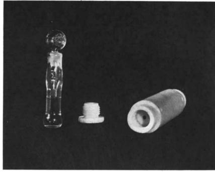
VOLUMETRIC FLASK with a capacity of 200 microliters (left) is used to develop solution for colorimetry in the spectrophotometer. The solution is removed from the flask with a pipette and put in an absorption cell (right). All the apparatus depicted in this article was photographed at the Socony-Vacuum Laboratories in Brooklyn, N. Y.
