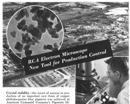
phthalocyanine blue pigment was achieved at American Cyanamid Company's Pigments Division through the use of the RCA Electron Microscope. Routine checks maintain particle size-help prevent crystal growth.
