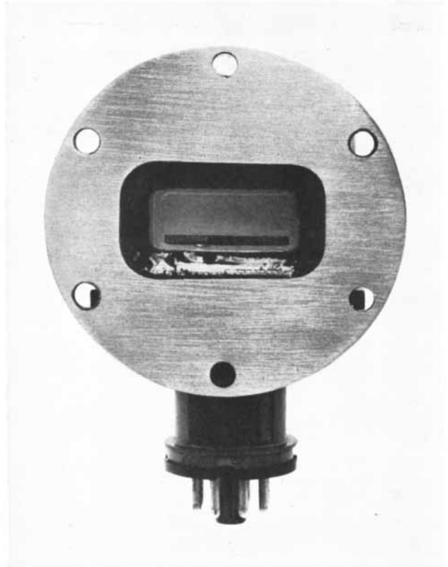
centimeters long. The oblong opening in photograph at right is coupled to a wave guide, the pipe used to conduct microwaves.
