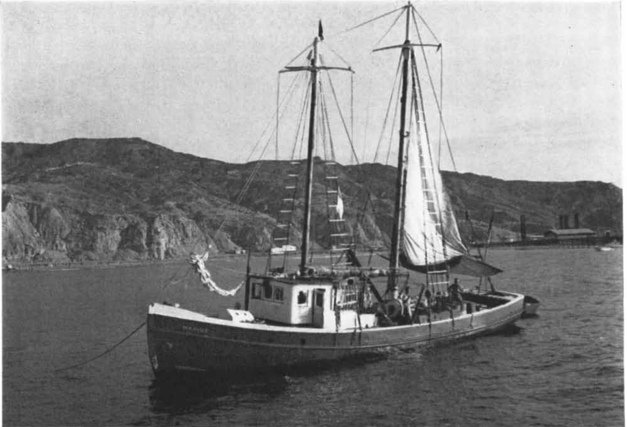
EXPEDITION BOAT was the 60-foot Marise . This former fishing craft was refitted for oceanographic purposes and sailed by the
