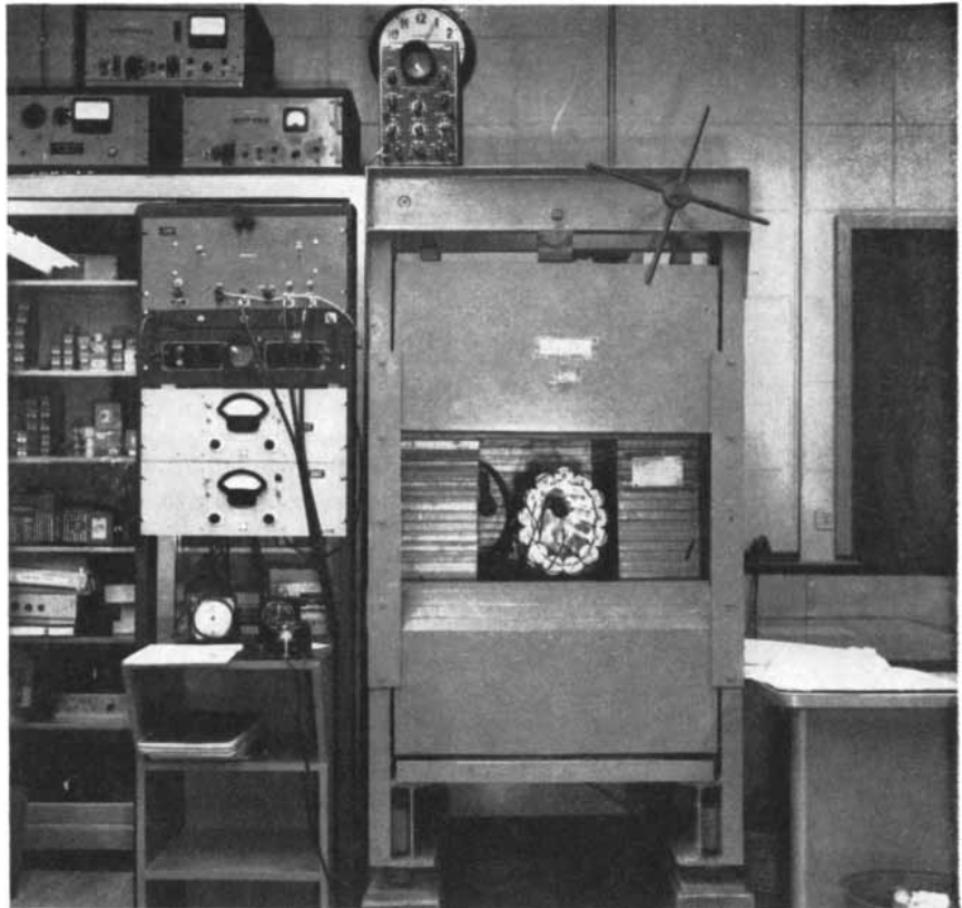
GEIGER COUNTER is used to measure the tritium content of water at the University of Chicago. The sample is placed within the array of Geiger tubes at right center. The tubes are heavily shielded against extraneous radiation. Door is lowered when counts are made.
