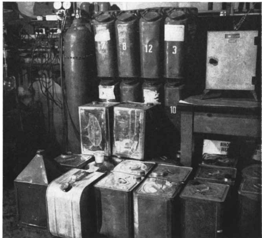
WATER SAMPLES are piled at the side of the University of Chicago laboratory. Some of the samples are rainwater, some river water and some lake water. Beneath the table at the right is a case of wine. The tritium in as little as a gallon can be measured accurately.
