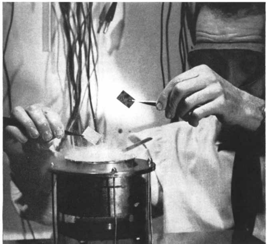
SMALL GENERATOR of the type illustrated at the upper left is demonstrated with two squares of steel. The clean piece of metal at left was dipped in the solvent only momentarily.
