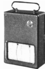
PORTABLE TEMPERATURE, HUMIDITY RECORDER Rugged, compact design. Ideally suited for use in small space and difficult locations. Provides convenient 3 x 5 charts for 10 or 30 hour records.
