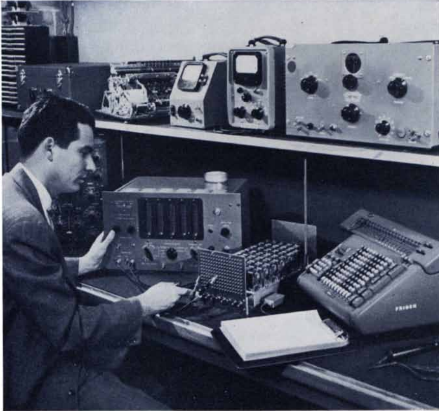
Electronic test instruments used daily at Friden include Hewlett-Packard oscillators, voltmeters, power supplies, electronic tachometers and the new, amazingly versatile -hp- electronic counters.
